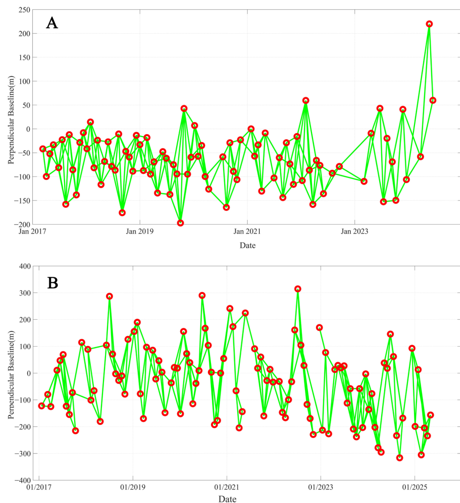
Figure 2. SAR data spatial baseline combination map ((A). Sentinel-1A data; (B). RADARSAT-2 data).
