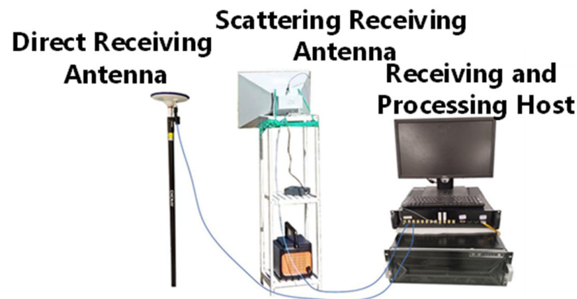
Figure 1. Diagram of GNSS-S Radar System.
