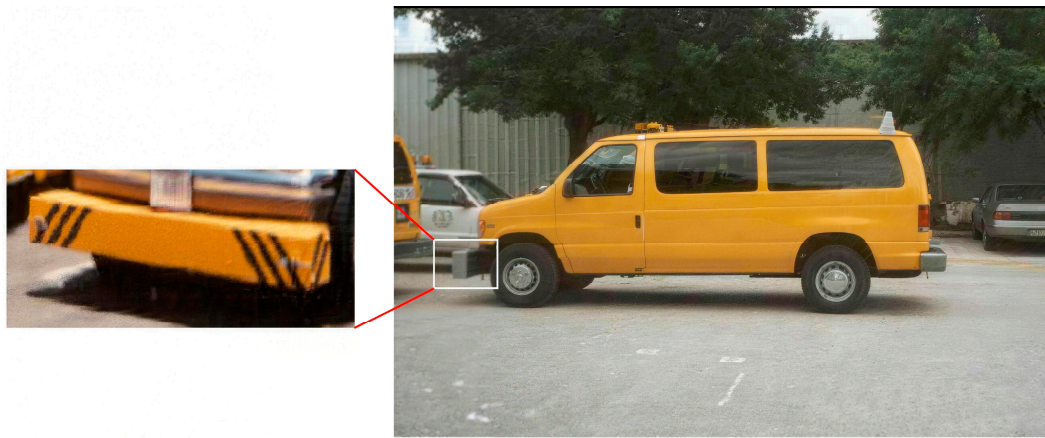
Figure 5. ICC MDR 4086L3 vehicle-mounted laser profilometer [48].
