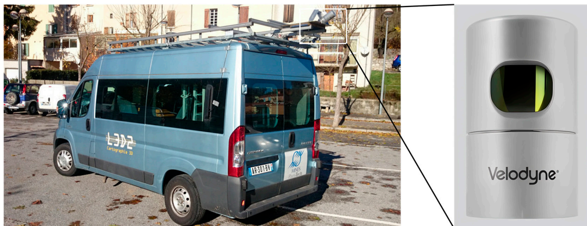
Figure 7. L3D2 vehicle-mounted laser scanning system [50].
