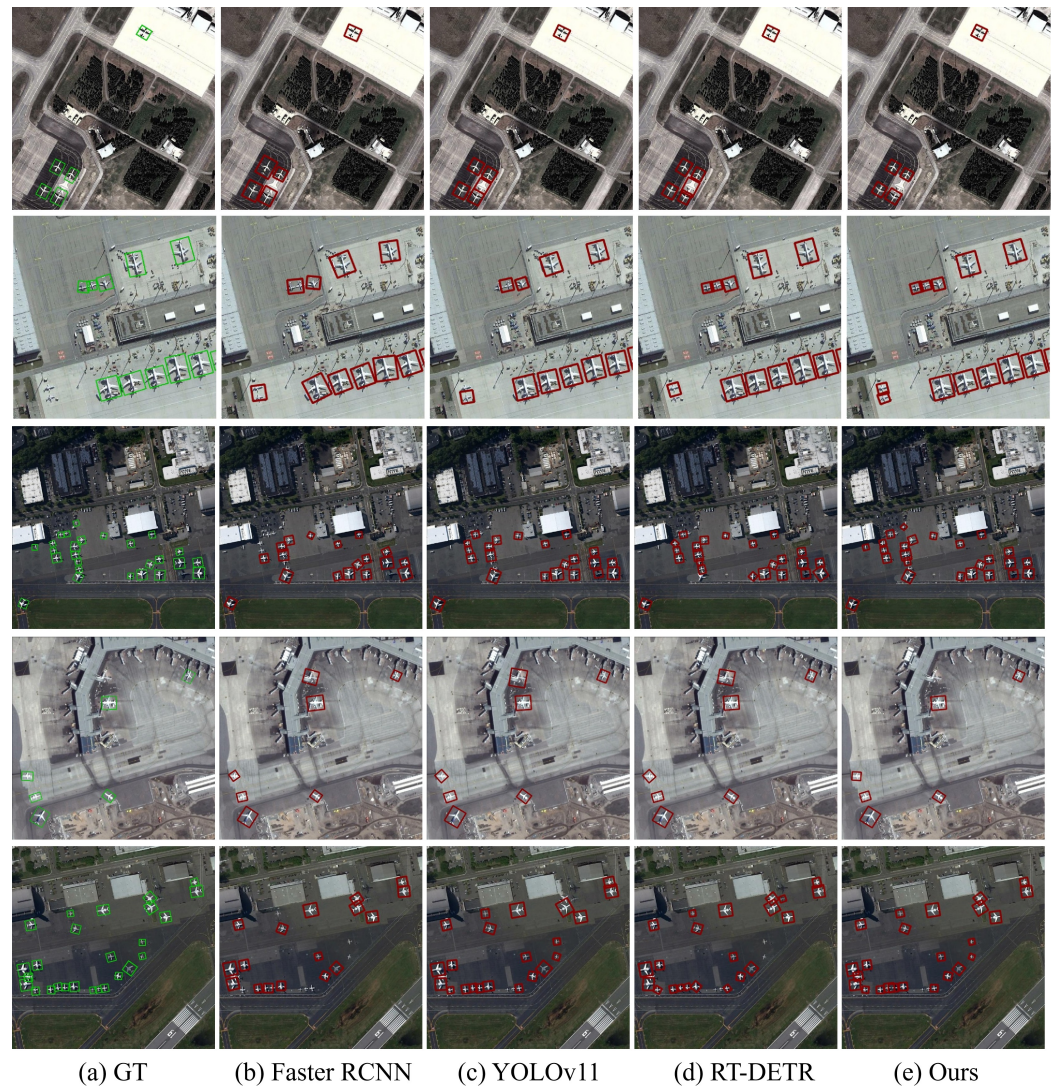
Figure 8. Visual comparison of detection results on the UCAS-AOD dataset. (a) Ground truth, (b) Faster R-CNN, (c) YOLO11, (d) RT-DETR, (e) SFSMamba-DETR. Green boxes denote ground-truth annotations, and red boxes denote model predictions. SFSMamba-DETR achieves more precise localization especially for small and overlapping targets.
