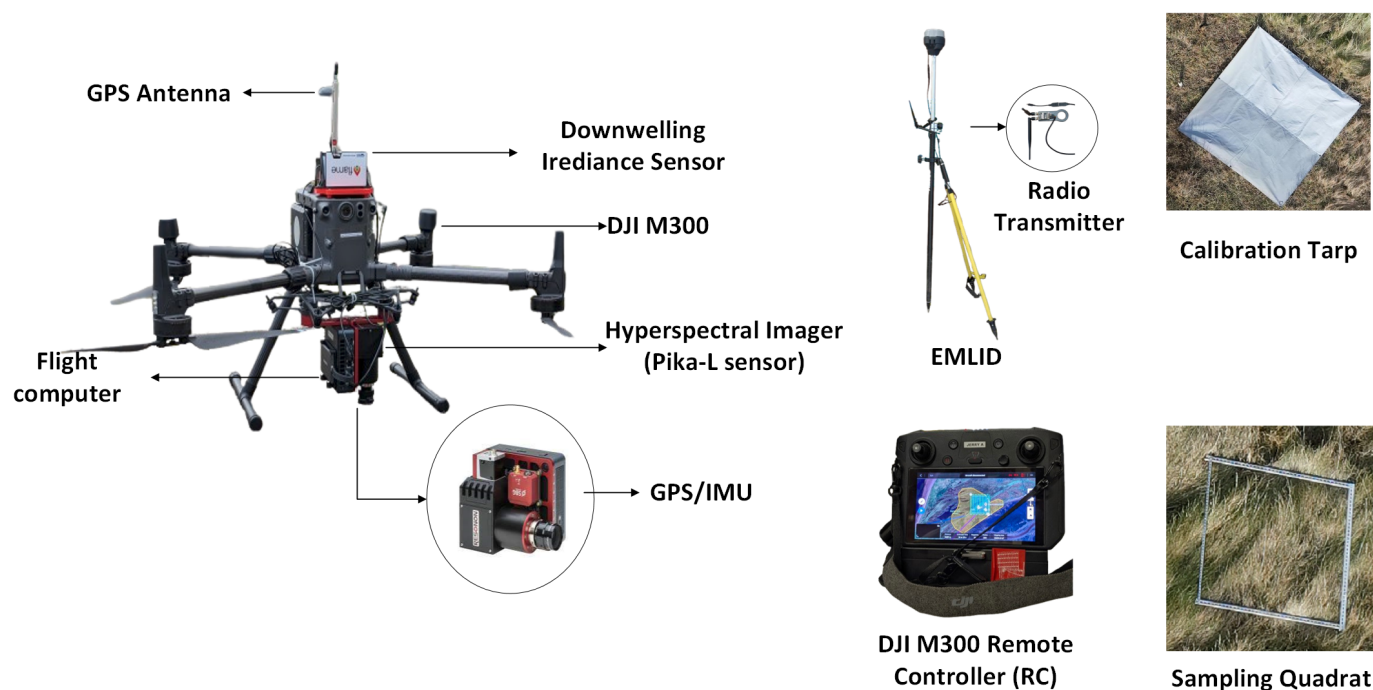
Figure 3. Experimental setup for hyperspectral data acquisition, including the DJI M300 UAV equipped with a Resonon hyperspectral imager, Emlid GNSS receiver, sampling quadrat, and calibration tarp.
