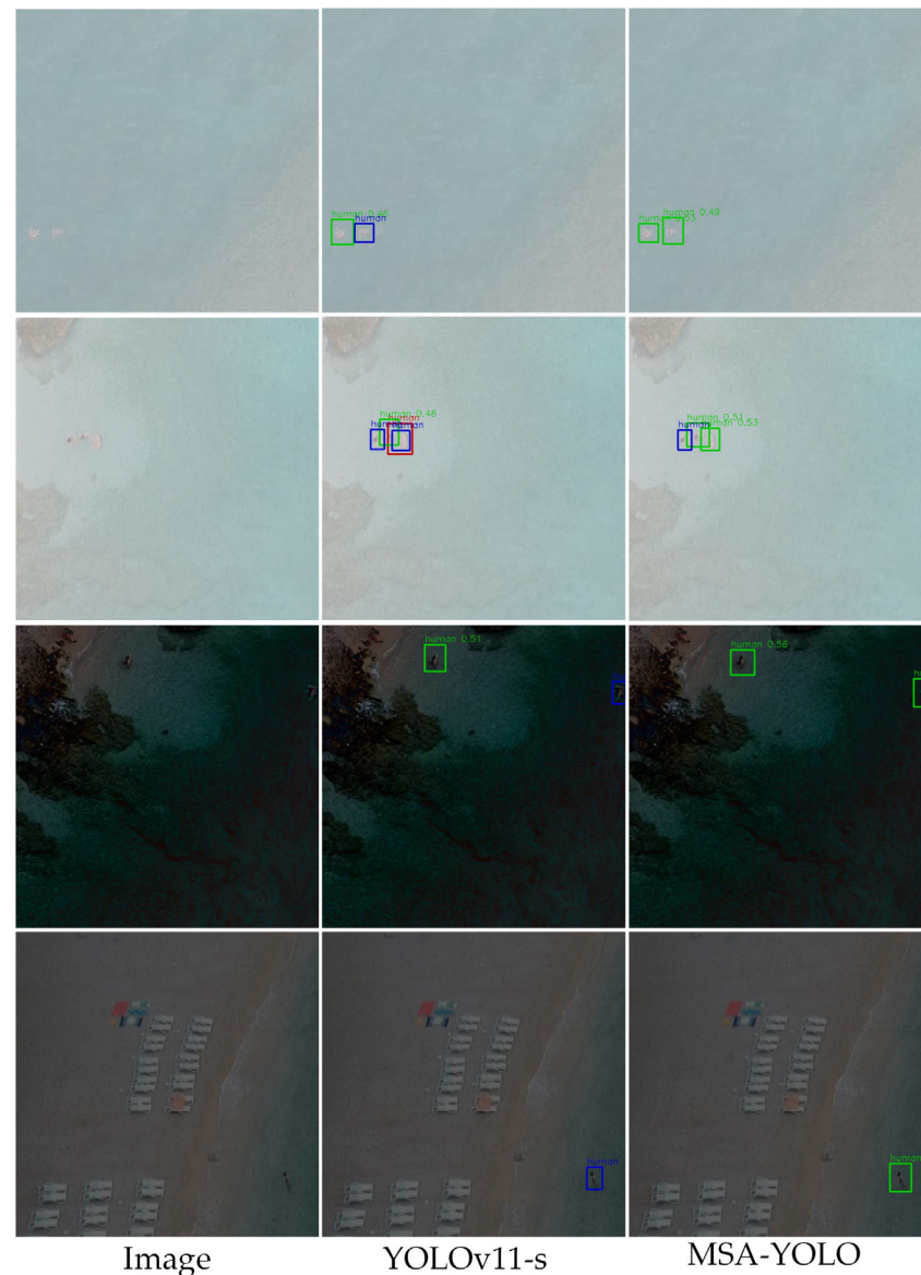
Figure 15. Comparison of small object detection under low-visibility conditions.
