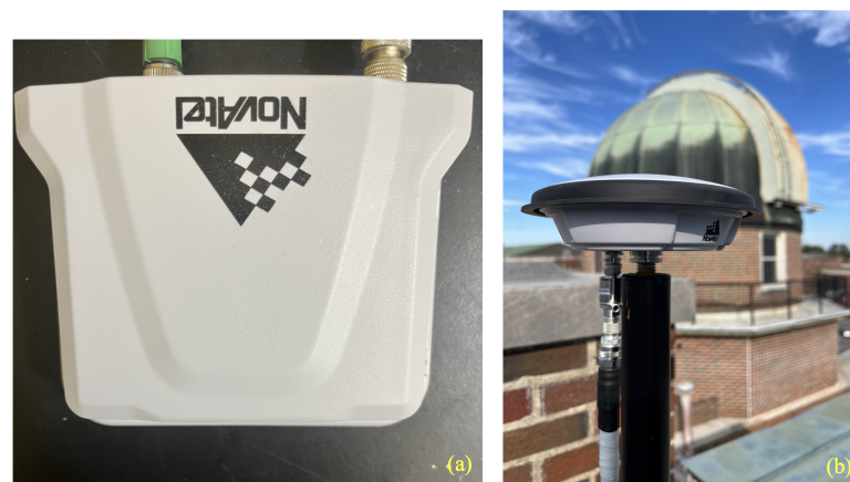
Figure 7. Experimental setup for the static scenario (a) Novatel receiver inside the lab and (b) fixed Novatel antenna shown in the foreground of the rooftop telescope at UA Physics and Astronomy.
