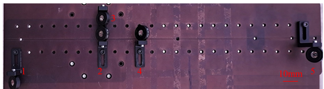
Figure 5. A multi-cone combination located at a distance of 4.3 km. The numbers 1–5 represent the serial numbers of the optical corner cube reflectors mounted on the metal plate.
