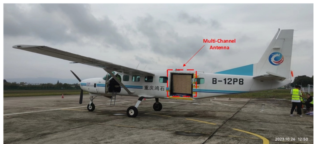
Figure 9. Airplane mounted with multi-channel SAR system.
