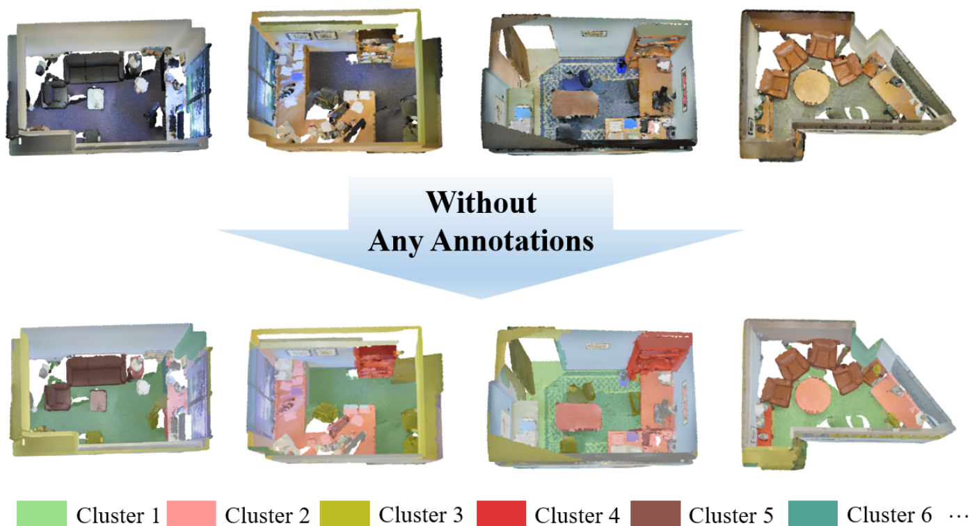
Figure 1. From raw point cloud data, our framework is designed to identify meaningful segments automatically without any supervisory signals. Different color blocks indicate distinct semantic clusters generated by the proposed method.
