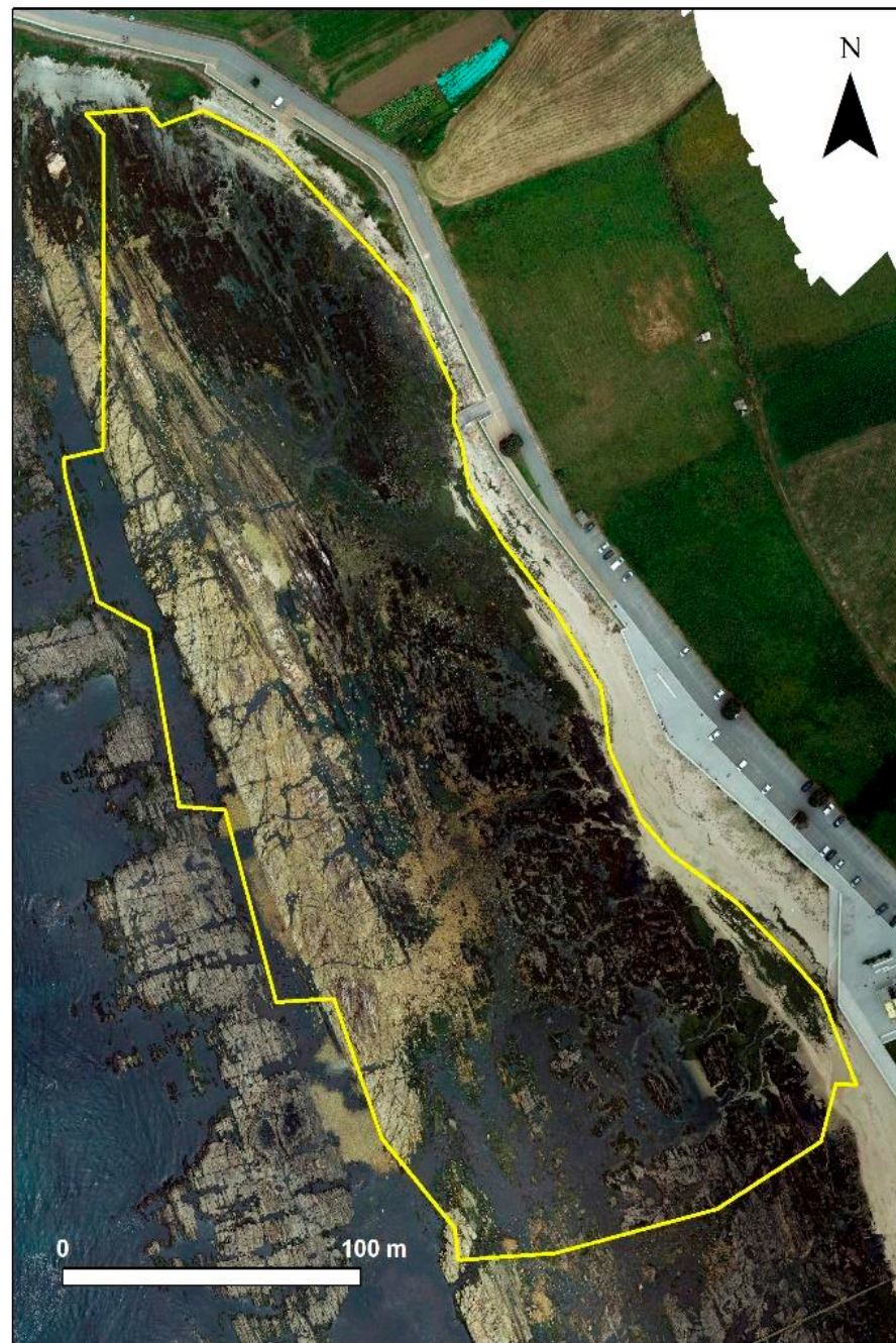
Figure 3. Orthomosaic of the intertidal area near Viana do Castelo ( 41^{\circ}41'45.6''\text{N} , 8^{\circ}51'10.8''\text{W} ), used for the determination of vegetation cover and the selection of VI (the yellow polygon delimits the area surveyed with a multispectral camera).
