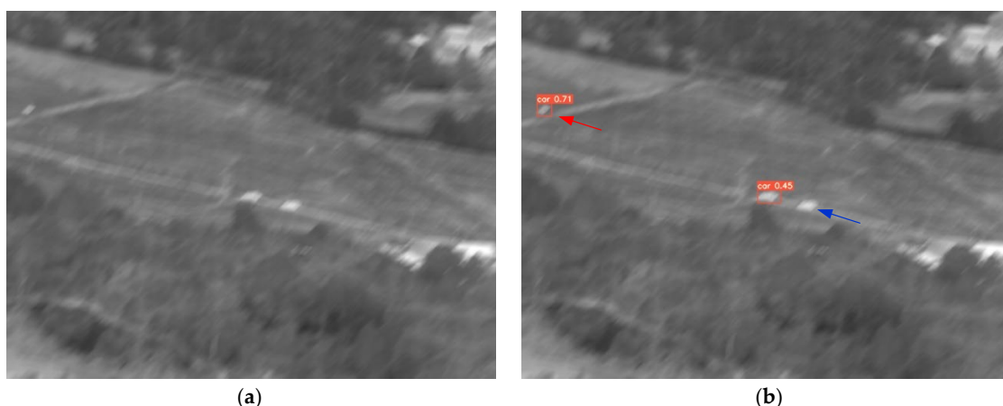
Figure 1. Poor visual quality and inadequate detection results of low-quality infrared images acquired from UAV platforms. (a) Acquired low-quality images; (b) Object detection results, where red arrows indicate false detections and blue arrows indicate missed detections.
