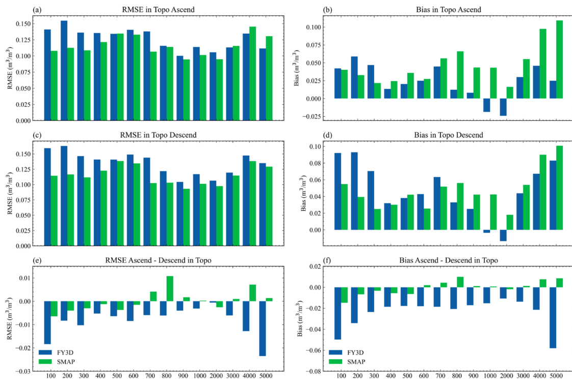
Figure 3. The average RMSE (left) and bias (right) between FY3D (first line) and SMAP (second line) soil moisture compared to that of the in situ results at different altitudes during the ascending (top) and descending orbits (middle), and the difference between ascending and descending orbits (bottom, ascending–descending orbits).
