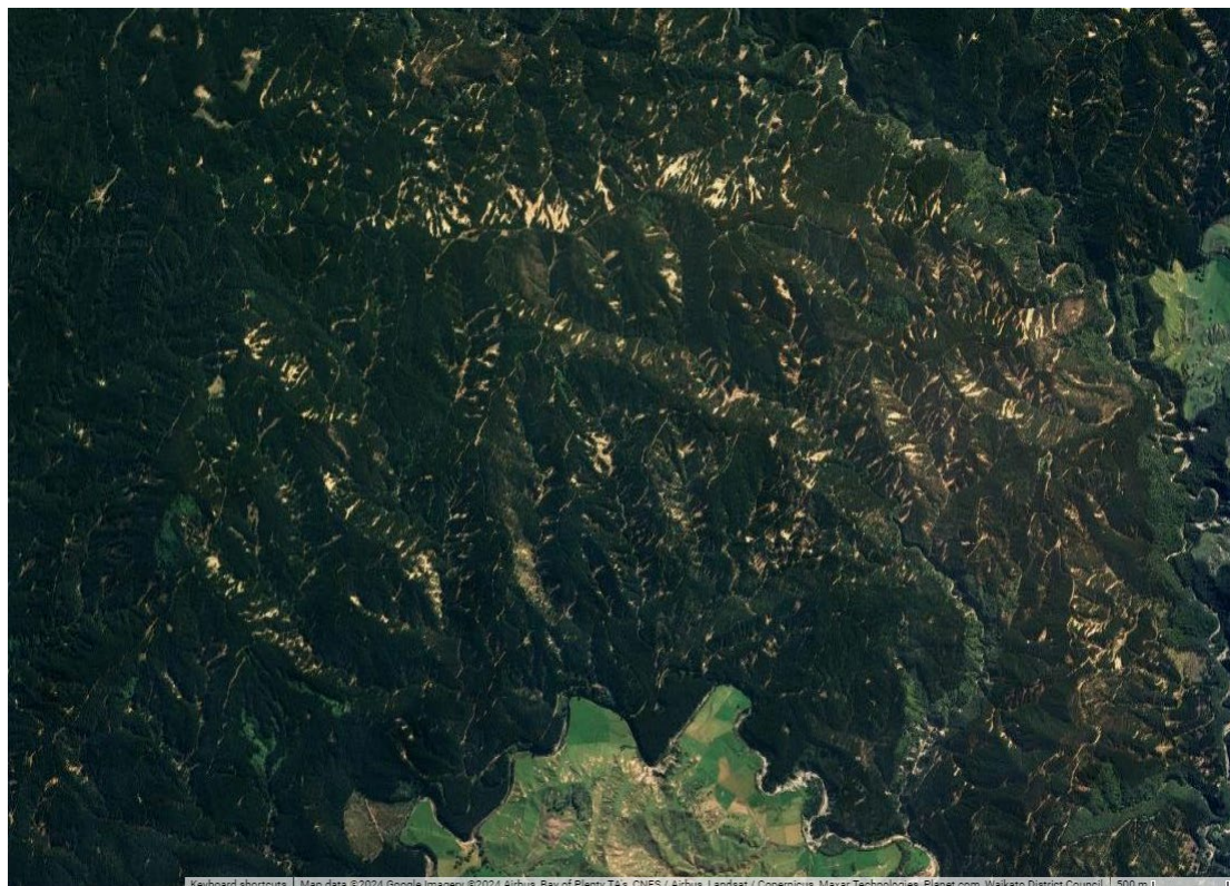
Figure 16. Screenshot from Google Earth Engine of the satellite base map for the region shown in Figure 14. The landslides shown here are relatively shallow and mainly located within a commercial pine forest plantation.
