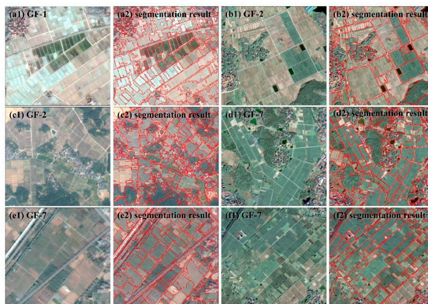
Figure 5. Visual examination of multi-scale segmentation result of GF-1, GF-2, and GF-7 imagery using Google Earth images. (a1) shows the original GF-1 image; (b1,c1) are original GF-2 images; and (d1,e1,f1) are original GF-7 images. Panels a2 through (f2) present the corresponding segmentation results for each of the above images.
