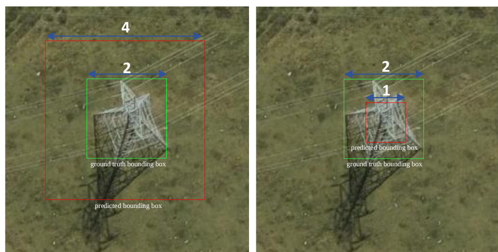
Figure 8. Two different bounding box regression results. The green boxes represent ground-truth bounding boxes with a length of 2 units. The red boxes represent predicted bounding boxes, with a length of 4 units in the left image and 1 unit in the right image.
