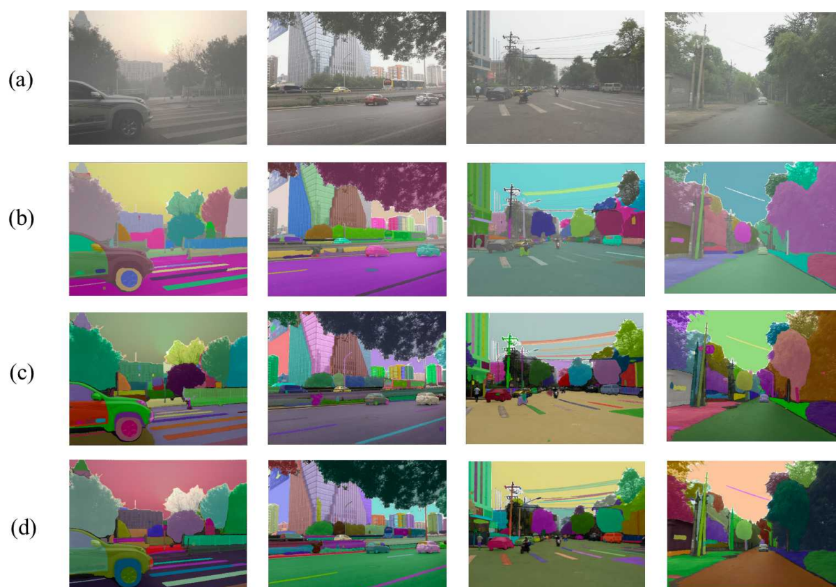
Figure 11. Visualization of the impact of the WRPM on segmentation accuracy. (a) The street view image captured under harsh weather conditions. (b) The segmentation result obtained without any preprocessing. (c) The segmentation result after applying the WRPM. (d) The ground truth for comparison.
