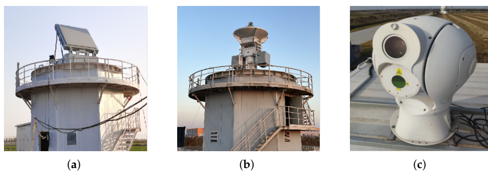
Figure 1. Experimental equipment. (a) High-resolution phased-array scanning radar. (b) High-resolution tracking radar. (c) Optical imaging system.
