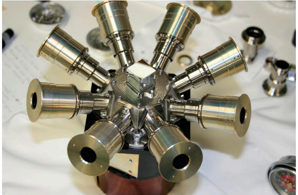
**Figure 6.** Fully assembled ARGOS instrument prepared for radiometric testing. The small reference cube in the center of the hub is used for optical alignment. This image was taken before the addition of thermal blankets for flight operations.
