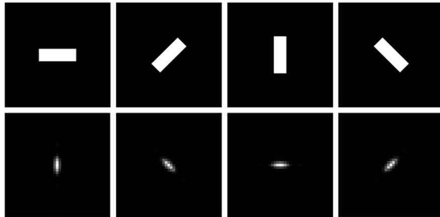
**Figure 2.** Rectangular pupils with different rotation angles and their point spread functions:  $0^\circ$ ,  $45^\circ$ ,  $90^\circ$ , and  $135^\circ$ , from left to right.
