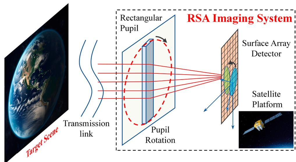
**Figure 1.** Imaging principle of the rotating synthetic aperture (RSA) system. Blue arrows represent the coordinate axes of the detector plane, while black arrows indicate the rotation of the pupil.
