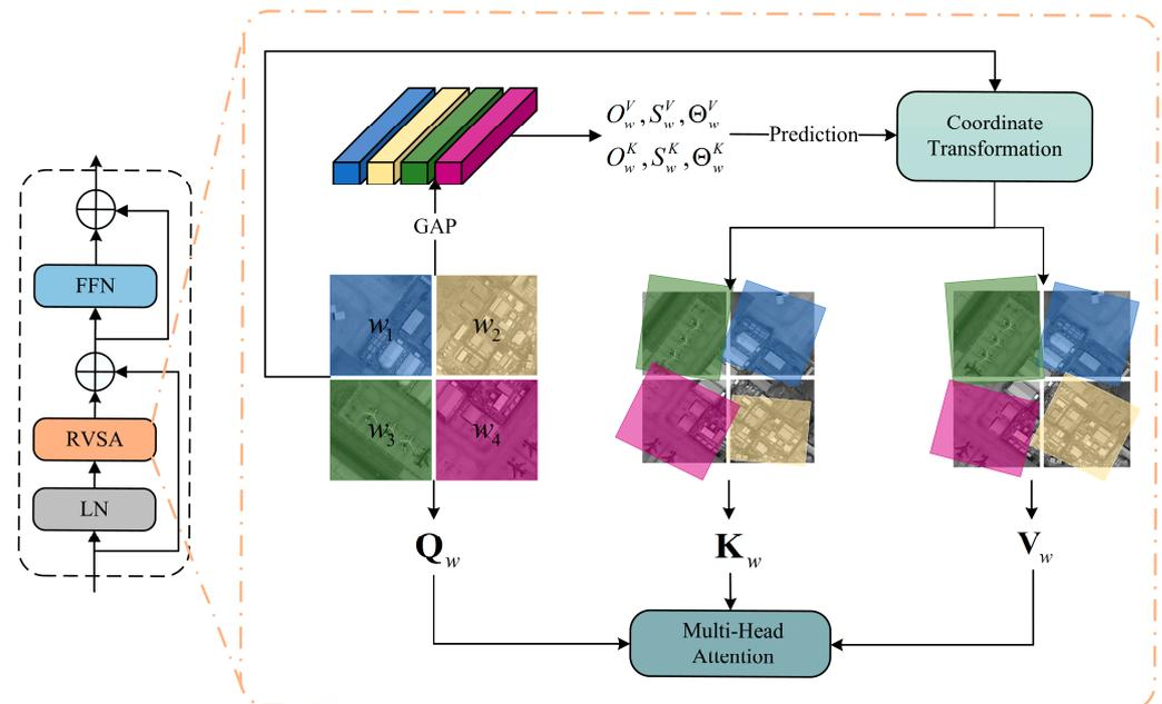
**Figure 6.** Illustration of rotated varied-size multi-head attention.
