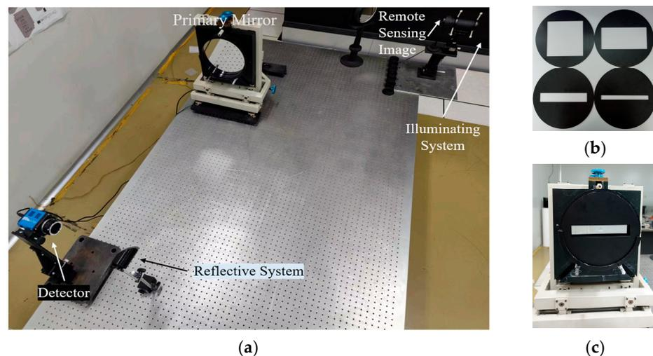
**Figure 9.** (a) Semi-physical imaging experiment platform; (b) rectangular pupil optical elements; (c) the primary mirror with a rectangular pupil optical element [44].
