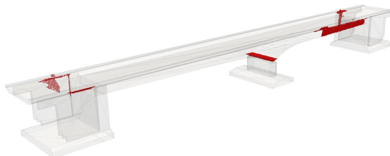
**Figure 13.** Uninspectable points of the railway bridge before the algorithm. Note that non-visible points below the surface have already been removed and are not considered in this representation. Uninspectable points are located at both ends of the bridge due to dense vegetation and at the middle pole.
