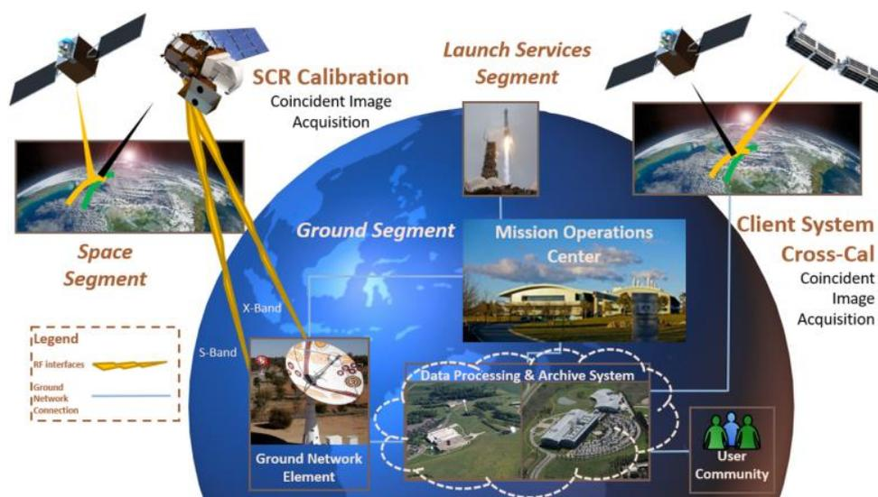
**Figure 9.** Schematic illustration of key elements in the notional SCR system architecture with captions. (Credit: USGS for graphics and captions).
