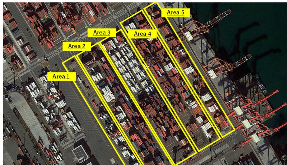
**Figure 2.** Example of detection area set in a container yard.
