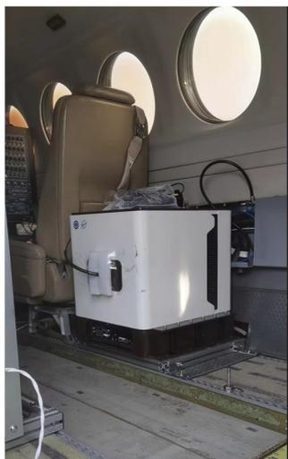
**Figure 4.** Actual installation of imaging differential optical absorption spectroscopy (IDOAS) equipment in the aircraft cabin.
