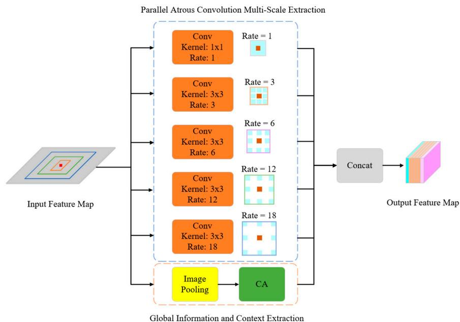
Figure 4. ASPP+ module structure.
