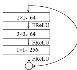
**Figure 6.** Bottleneck structure of ResNet50.
