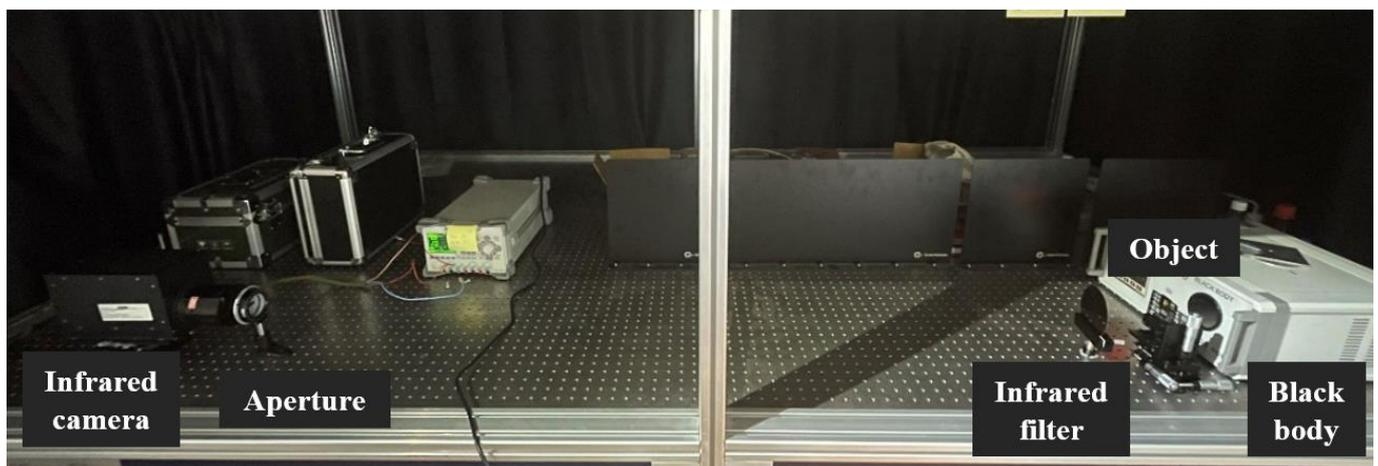
Figure 7. Experimental setup for aperture-coded Fourier ptychographic imaging.
