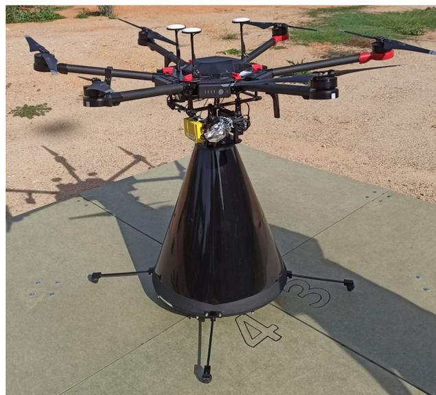
**Figure 7.** Image of a field experiment with the optical detection system already integrated within the unmanned aircraft DJI Matrice 600 Pro.
