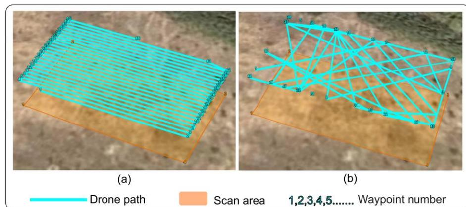
**Figure 18.** Schematics of scan patterns that can be generated by the ground control station during flights.
