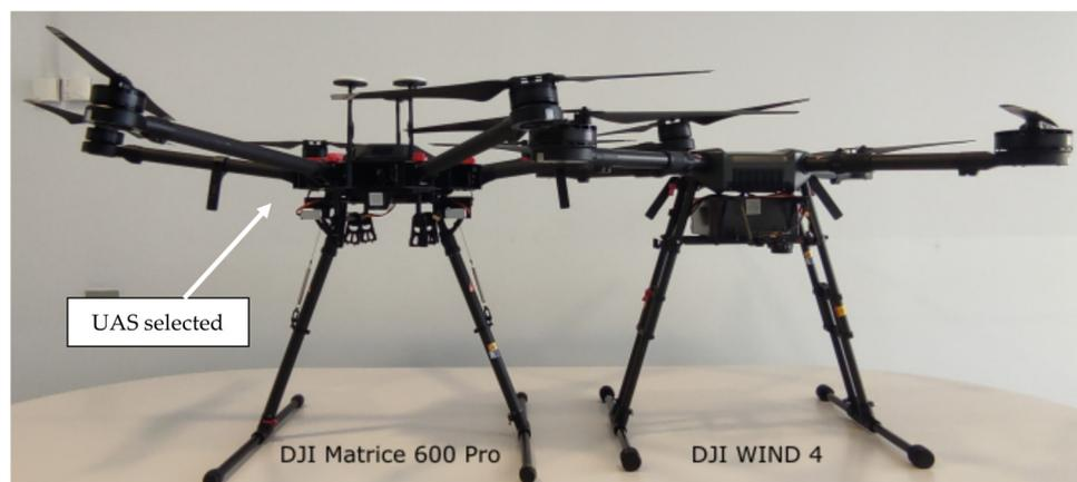
**Figure 5.** Pictures of the two unmanned aircraft systems evaluated to be used for the mounting of the optical system to remotely detect alpha particles. The DJI Matrice 600 Pro was finally used in this study.
