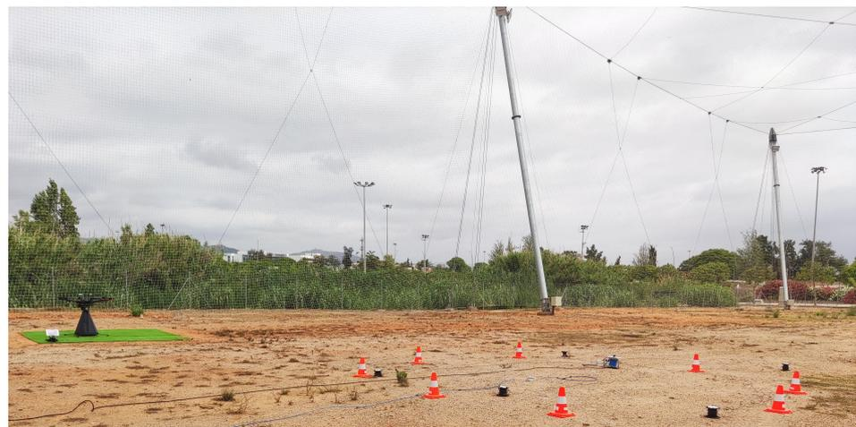
**Figure 21.** A picture of a typical configuration used for test flights carried out at the DroneLab of the Technical University of Catalonia. The five LED sources are the black cylinders located on the soil.
