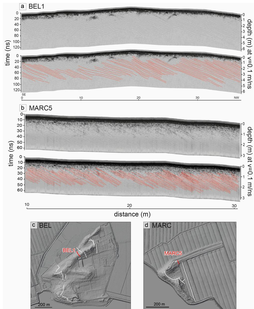
**Figure 14.** (a) BEL1 and (b) MARC5 radargrams with highlighted clinostratification. On the bottom, the location in Belvedere (c) and San Marco (d) of the highlighted radargrams (in red) and the other GPR lines (in white).
