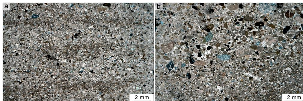
**Figure 11.** Thin sections of sample Muson27 in crossed-polarized light. See Figure 10 for orientation of the sample. (a) The darker layers consist of finer grains; (b) particular of the transition from a layer of fine sands (**bottom**) to coarser sand and fine gravel (**top**).
