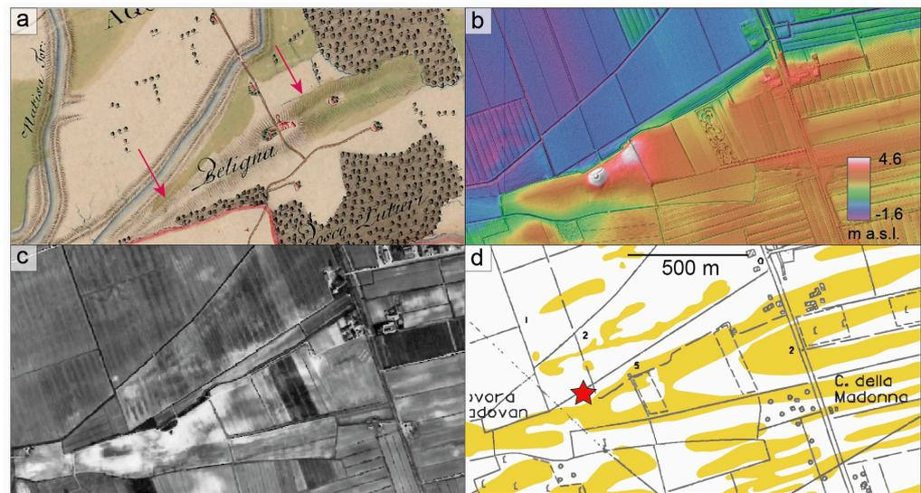
**Figure 8.** Area of Beligna, an example of integration of different data. (a) Historical cartography with red arrows indicating the slopes of the dunes' ridges; (b) DTM; (c) aerial photos (1993) (d) reconstruction of the planar morphology of the dunes (in yellow). The red star indicates the location of BLG1 borehole.
