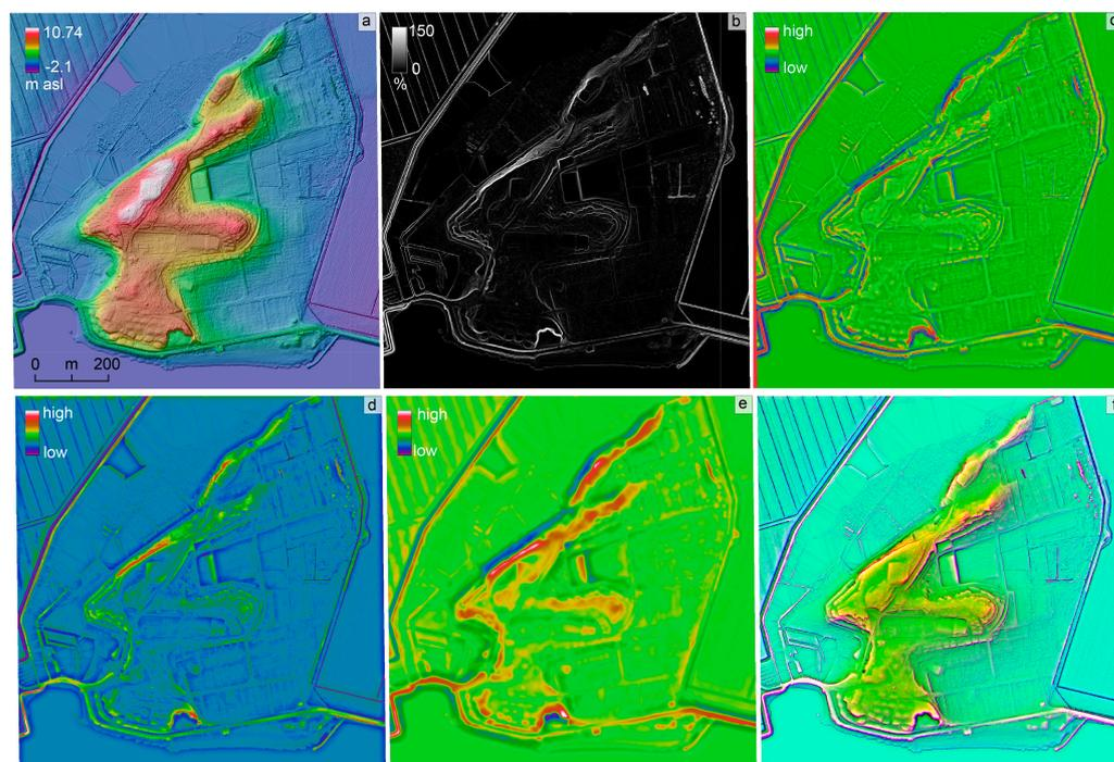
**Figure 3.** Elaborations of DTMs in the area of Belvedere Pineta Camp Ground (Centenera). (a) DTM and hillshading; (b) slope; (c) simple local relief model (SLRM); (d) local dominance; (e) multi-scale relief model (MSRM); and (f) principal component analysis of previous elaborations in RGB = pc1–pc2–pc3 composite.
