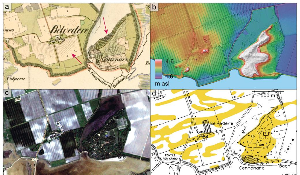
**Figure 7.** Area of Belvedere, an example of integration of different data. (a) Historical cartography with red arrows indicating the scarps of the dunes' ridges; (b) DTM; (c) satellite imagery (Planet: visible bands); (d) reconstruction of the planar morphology of the dunes (in yellow).
