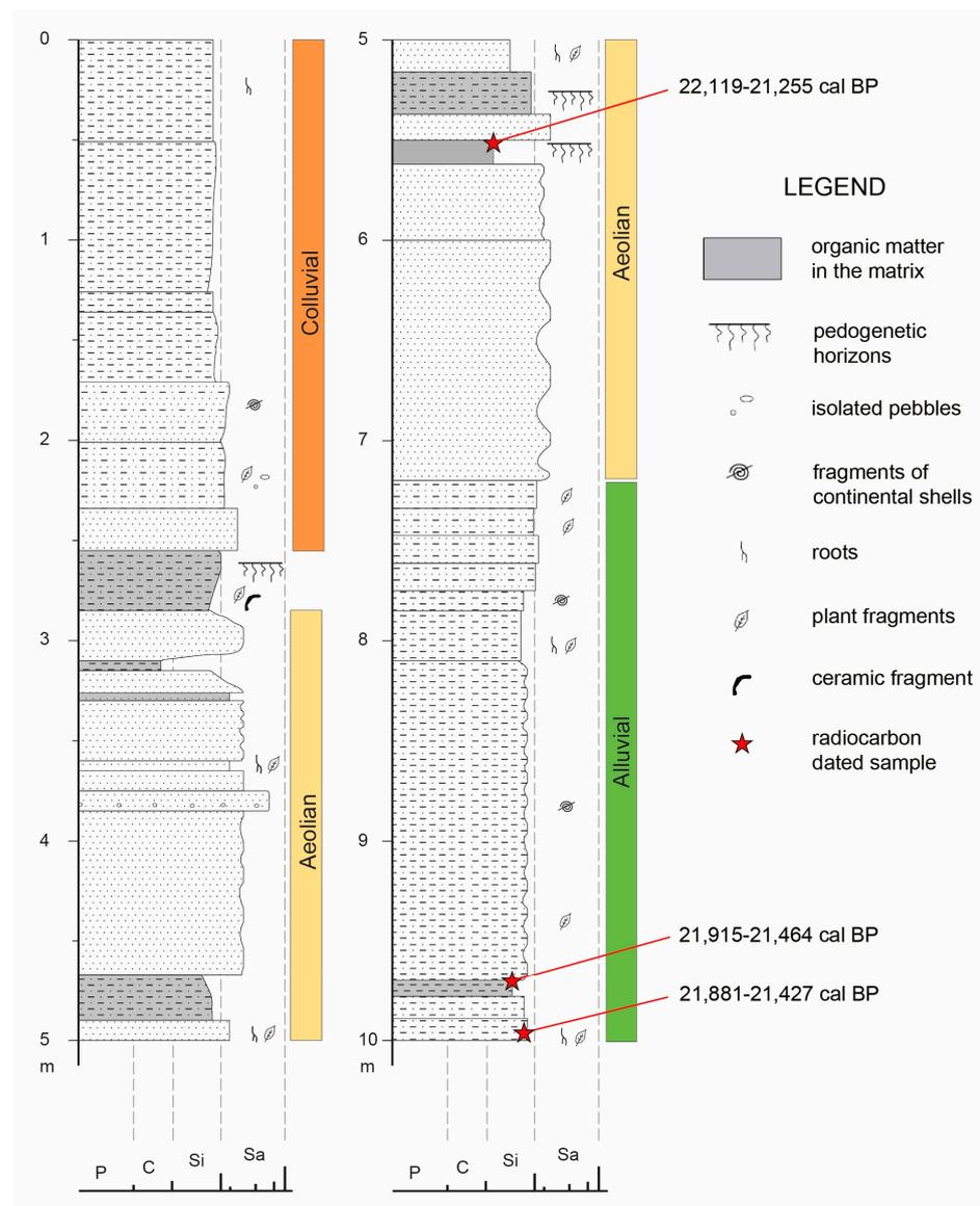
**Figure 13.** Stratigraphic log of the first 10 m of the core BLG1. Radiocarbon dates are calibrated (cal BP), as reported in Table 4.
