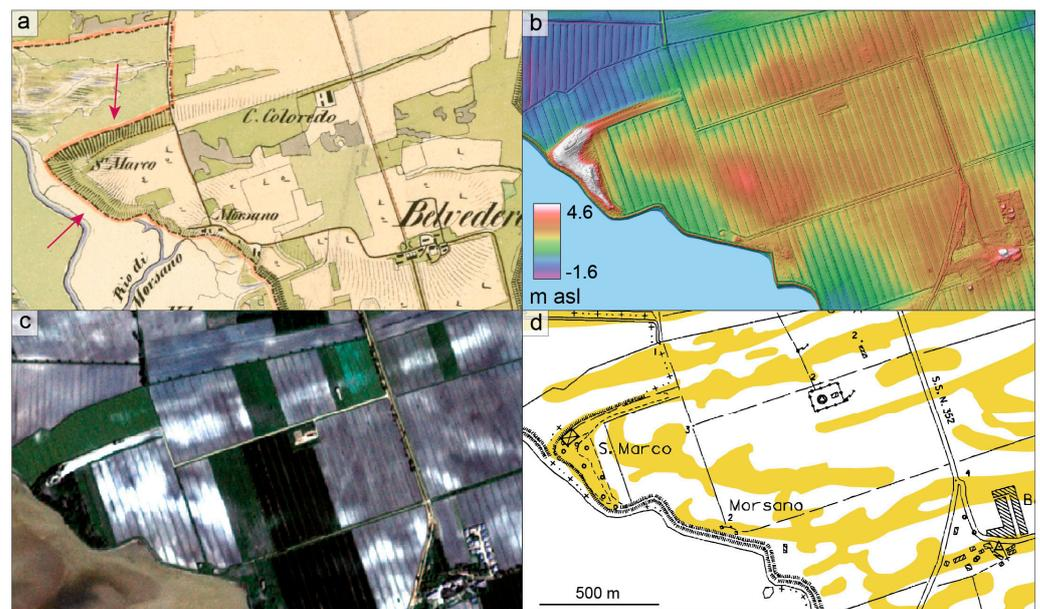
**Figure 6.** Area of San Marco, an example of integration of different data. (a) Historical cartography with red arrows indicating the slope of the dune ridges; (b) DTM; (c) satellite imagery (Planet: visible bands); (d) reconstruction of the planar morphology of the dunes (in yellow).
