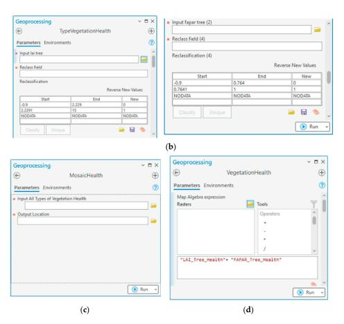
**Figure 8.** Vegetation health toolset consists of (**a**) mask tool for masking each type of vegetation, (**b**) TypeVegetationHealth tool for classifying healthy and stressed vegetation based on LAI and FAPAR, (**c**) VegetationHealth for combining vegetation health based on LAI and FAPAR, and (**d**) MosaicHealth for combining all types of vegetation health.
