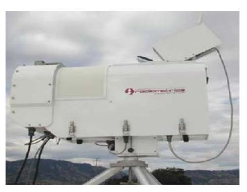
Figure 3. Photo of microwave radiometers produced by Radiometrics Corporation.
