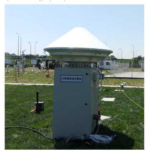
Figure 1. Photo of HMB-KPS millimeter-wave radar.
