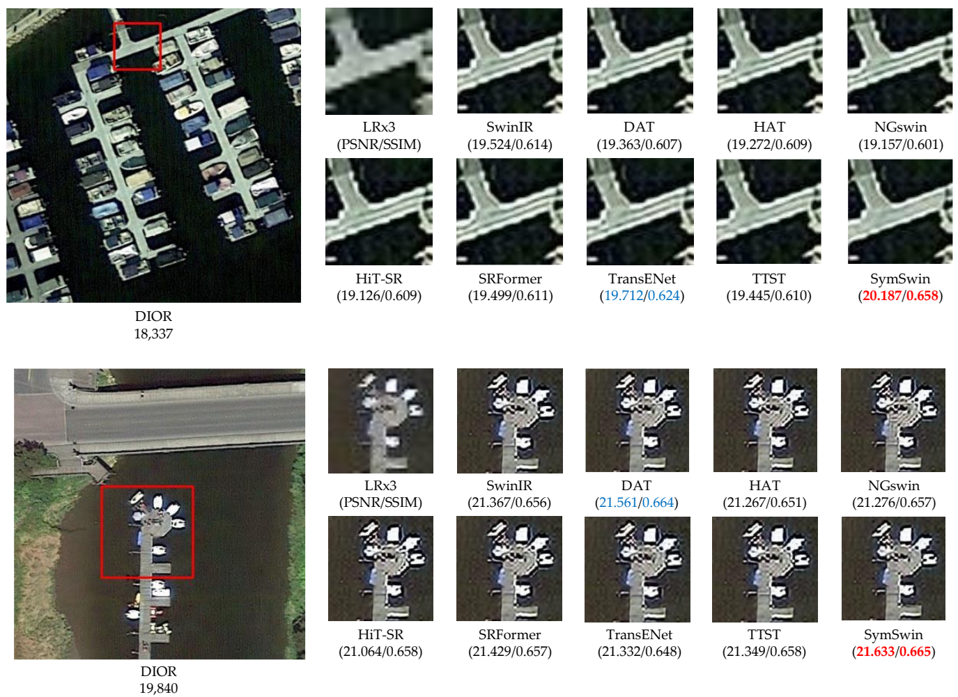
Figure 6. The visualization examples of the \times 3 super-resolution reconstruction inference results for the algorithms mentioned in the quantitative experiments on datasets NWPU-RESISC45 and DIOR. The values PSNR and SSIM are listed below each patch, the best performance is highlighted in bold red font and the second-ranked is highlighted in blue font. The inset on the right is a magnified view of the region enclosed by the red bounding box in the main image. Zoom in for better observation.
