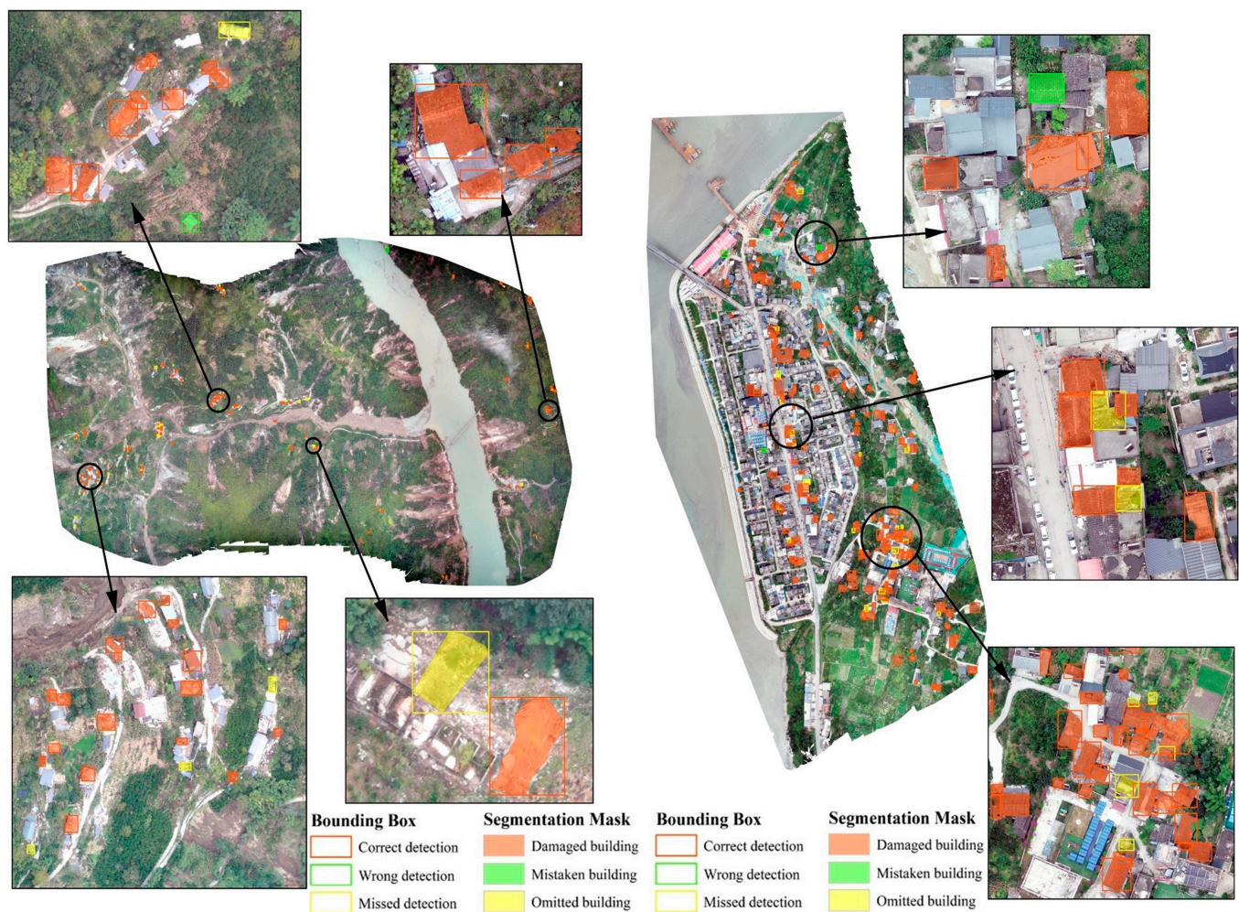
Figure 15. Results of damaged building classification in Wandong village and Detuo town (Figure 1B(f,g)). Red indicates correct detections, green indicates incorrect detections, and yellow indicates missed.
