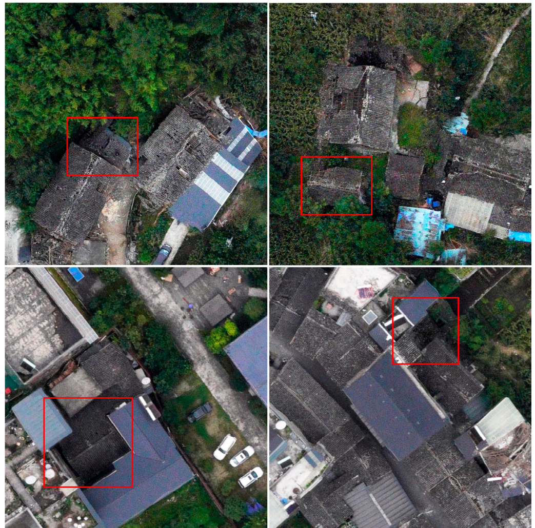
Figure 18. Examples of densely built-up areas. The red boxes indicate buildings with blurred contour information caused by shadows and occlusions.
