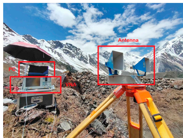
Figure 4. Physical diagram of the GB radar system.
