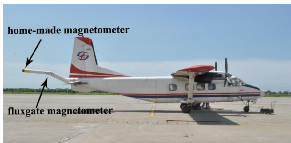
Figure 3. Photo of our aeromagnetic detection aircraft.
