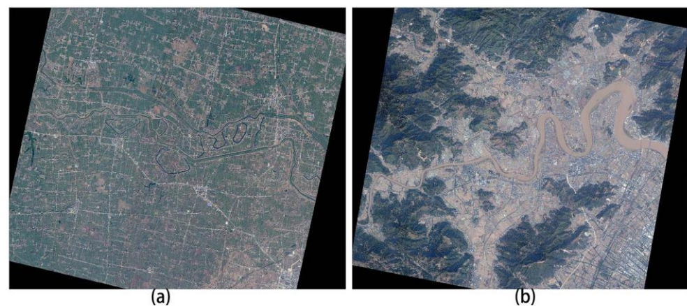
Figure 2. Remote sensing images acquired by satellite. Both images above have a resolution of 0.8 m. (a) shows a 27,844 \times 26,864 four-band remote sensing image of the farmland in Anhui Province, which can generate 3711 effective training images of 512 \times 512 pixels. (b) shows a 27,500 \times 26,760 four-band remote sensing image of the farmland in Zhejiang Province, which can generate 3655 effective training images.
