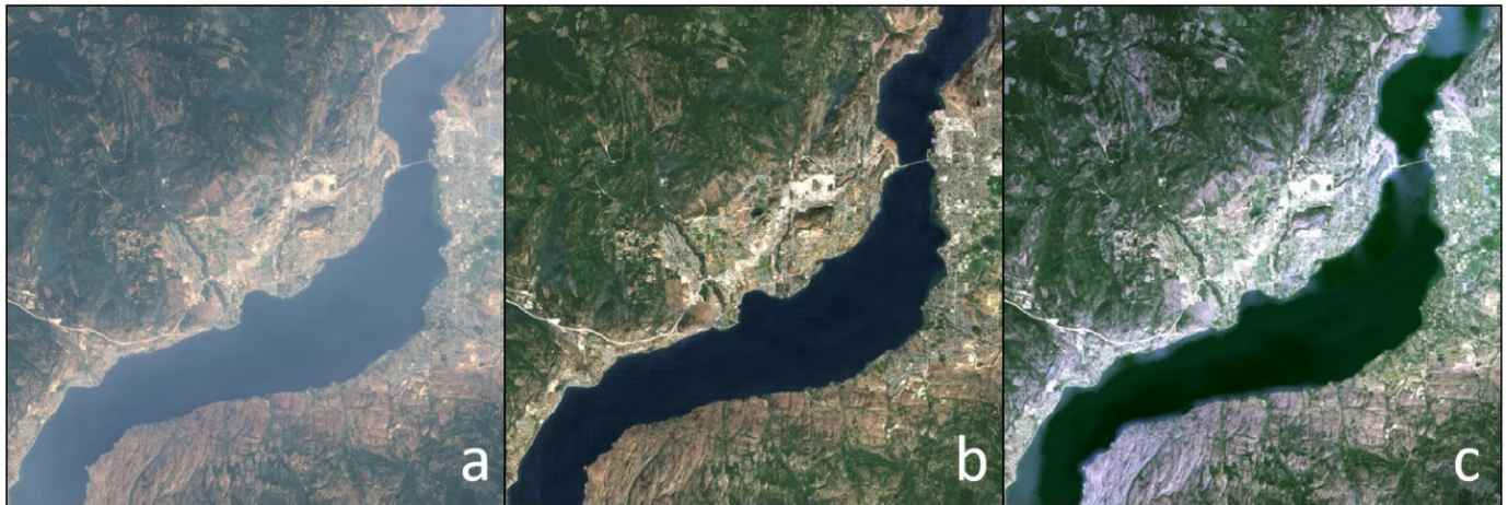
Figure 1. The quality of atmospheric correction can be judged by image clarity and color balance. Landsat-8 image of Kelowna, British Columbia, 8 August 2021, portrayed in true color: (a) uncorrected TOAR, (b) CMAC corrected, and (c) LaSRC corrected.
