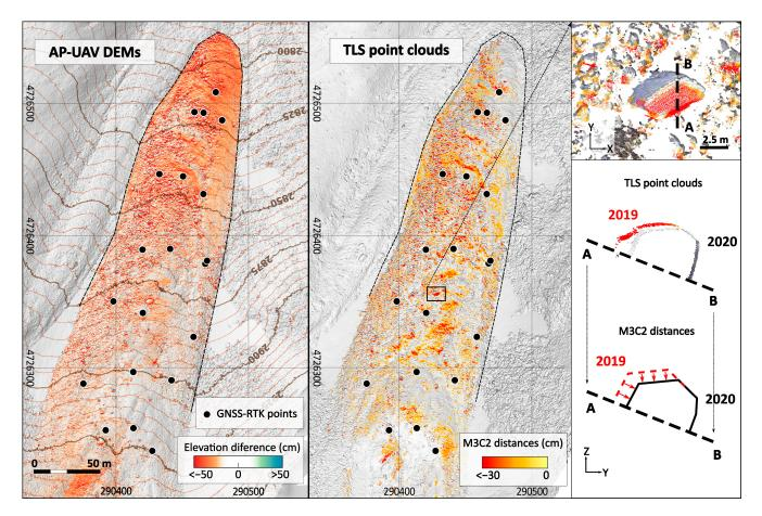
**Figure 8.** Surface changes of the La Paúl rock glacier between 2019–2020 (Coord. System ETRS89 UTM 30N). (**Left**) Significant vertical variations (LOD95%) determined through AP-UAV DEMs. AP-UAV hillshade DEM background. (**Right**) Significant 3D variations (LOD95%) determined through TLS point clouds. Shadowed TLS background.
