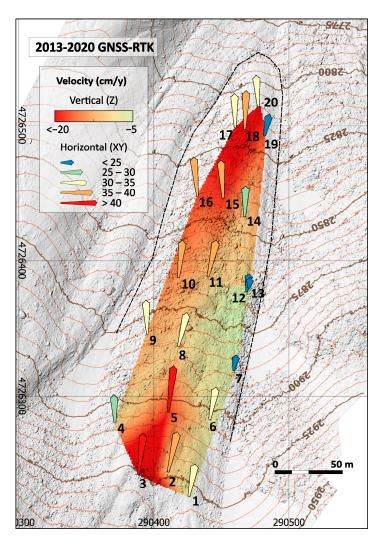
**Figure 7.** Annual horizontal and vertical surface velocities of the La Paúl rock glacier derived from GNSS-RTK measurements. Horizontal displacements scaled ×10. AP-UAV 2020 DEM elevation and hillshading background. Coord. System ETRS89 UTM 30N.
