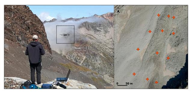
**Figure 4.** (Left) DJI Mavic 2 Pro UAV used in the photogrammetric flights of La Paúl in mid-flight (2019). (**Right**) Target locations (cross symbol) used in the photogrammetric flights on the rock glacier (2020). Orthomosaic from PNOA (CC-BY 4.0 scne.es).
