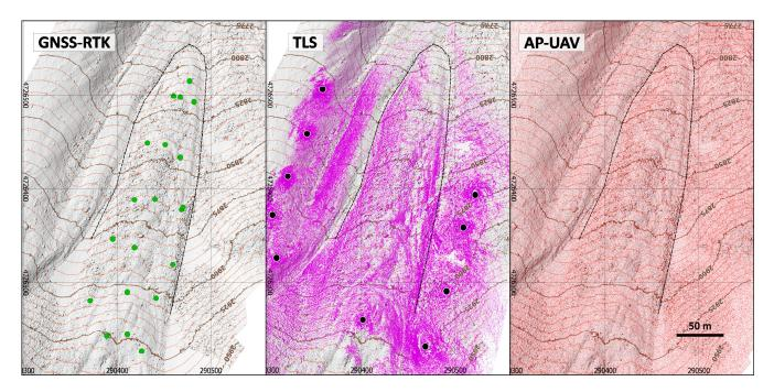
**Figure 5.** Points measured by GNSS-RTK (green), TLS (violet; black dots show scan locations), and AP-UAV (red) on La Paúl rock glacier in 2019. Hillshade background generated from DEM AP-UAV 2020. Coord. System ETRS89 UTM 30N.
