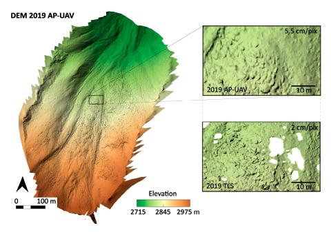
**Figure 6.** Elevation model derived from AP-UAV techniques in La Paúl rock glacier (2019), with surface details from AP-UAV and TLS DEMs.
