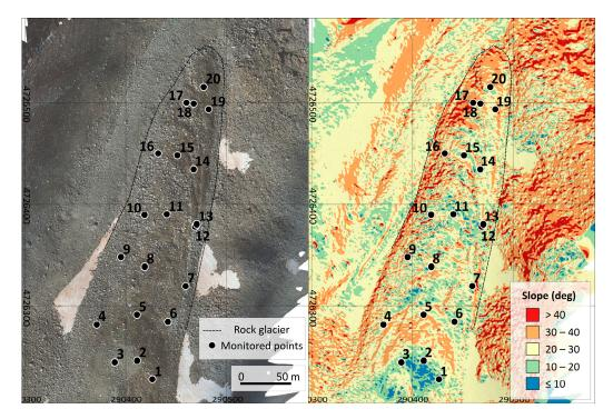
**Figure 2.** Location of the 20 singular points defined in the La Paúl rock glacier for monitoring by GNSS techniques (Coord. System ETRS89 UTM 30N). (**Left**) Orthomosaic from AP-UAV 2020. (**Right**) Slopes derived from the AP-UAV 2020 elevation model (resampled to 1 m resolution).
