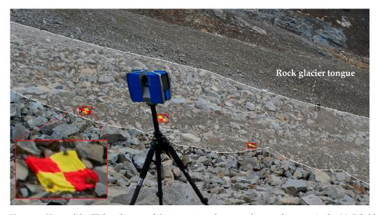
**Figure 3.** View of the TLS and some of the targets used to georeference the scans in the 2017 field campaign.
