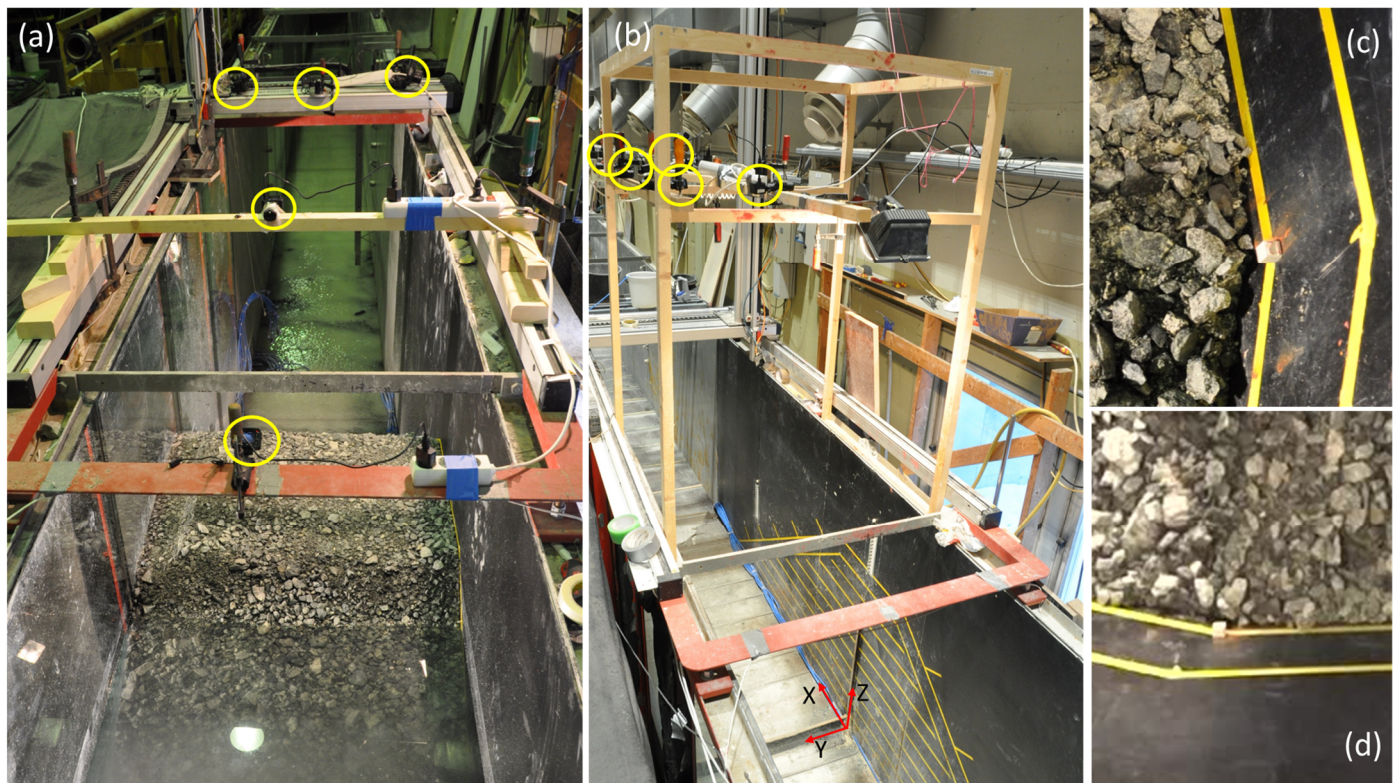
Figure 3. Camera rig setups (a) Model U1-U3 (b) Model U4-H3, camera locations indicated by yellow circles, coordinate system definition shown on (b) with red arrows and axis labels (c) shows DSLR image of a GCP cube (d) shows video frame of the same GCP cube.
