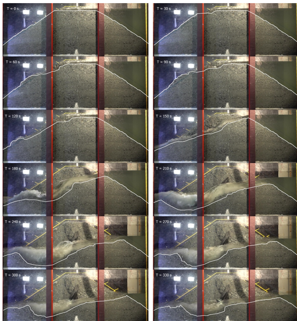
Figure 8. Side-view tracking of breach progression of model U4 (central core); direction of flow is right to left ; white line indicates traced solid surface.
