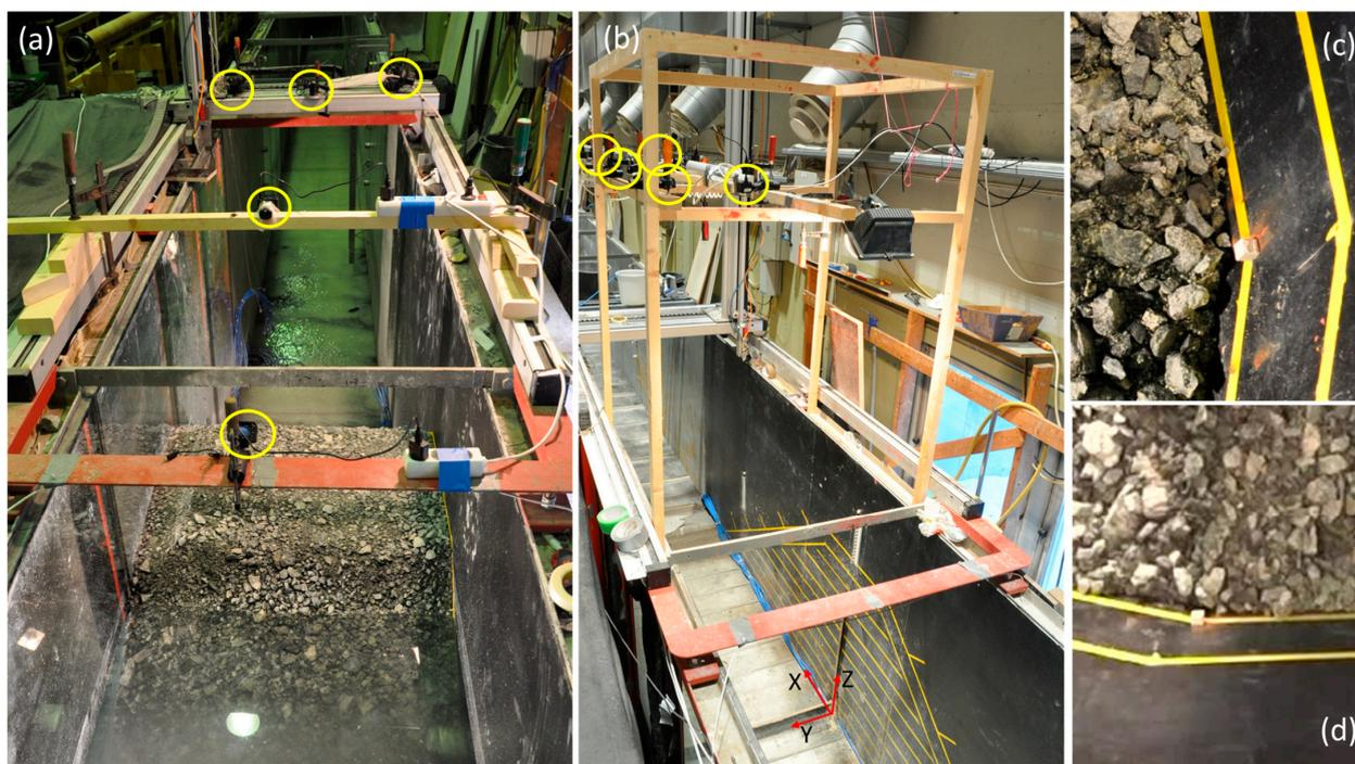
**Figure 3.** Camera rig setups (a) Model U1-U3 (b) Model U4-H3, camera locations indicated by yellow circles, coordinate system definition shown on (b) with red arrows and axis labels (c) shows DSLR image of a GCP cube (d) shows video frame of the same GCP cube.
