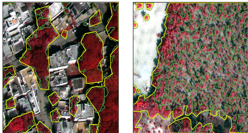
Figure 2. Illustration of the two different qualities of delineating tree crowns: an urban (left) and a rural (right) environment. Yellow denotes rough delineations and green denotes accurate delineations of tree crowns.
