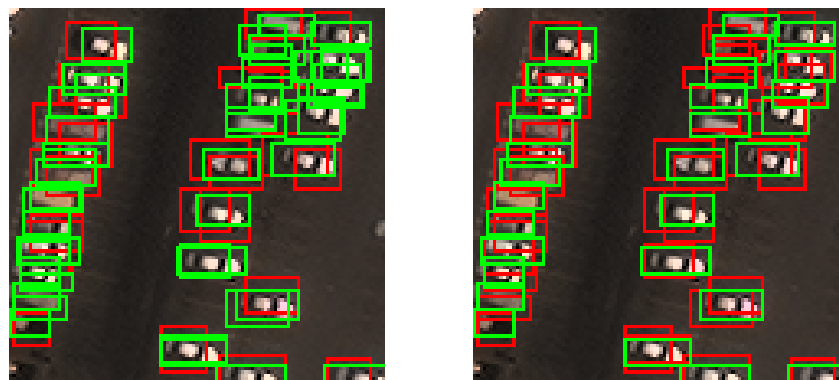
Figure 5. The green bounding boxes are positive samples that have been assigned to vehicle ground truths, while red bounding boxes are negative samples that will not be trained in the bounding box regression training process. The left picture shows the positive samples assigned only by calculating IoU. In this case, we choose 0.7 as the IoU threshold. Every proposal which has IoU greater than the threshold is assigned to the ground truth with max IoU. The right picture shows the positive samples assigned by the Density-assigner. In the dense area, only a single proposal is assigned to each ground truth as the positive sample. By contrast, positive samples assigned by the Density-assigner are of high quality, and poor proposal samples, which locate among several ground truths, are no longer assigned in this case.
