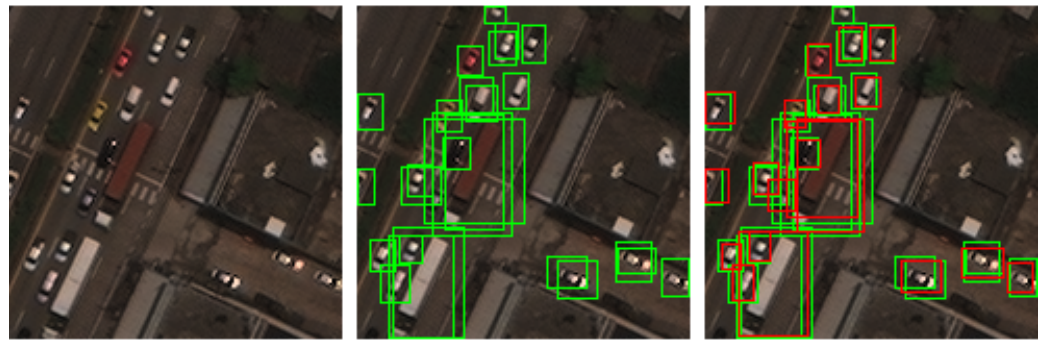
Figure 7. The visualization of proposals kept after traditional NMS and our proposed Scale-NMS. The left image is the original aerial image, the middle one is the result of traditional NMS with a threshold of 0.7, and the right one is the result from our proposed method with an NMS threshold from 0.7 to 0.85. The red bounding boxes are proposals kept in our method, which are supplements to the proposal list.
