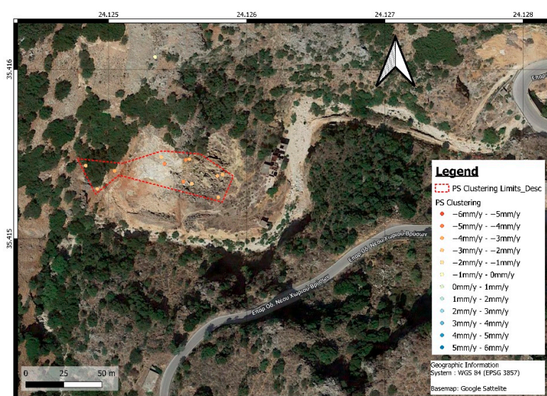
Figure 5. Identification of potential ongoing landslide events in the entrance of the Macheri village [36].
