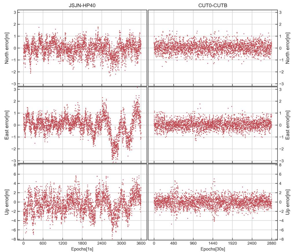
**Figure 5.** The time series of DD code positioning errors for JSJN–HP40 (left) and CUT0–CUTB (right).
