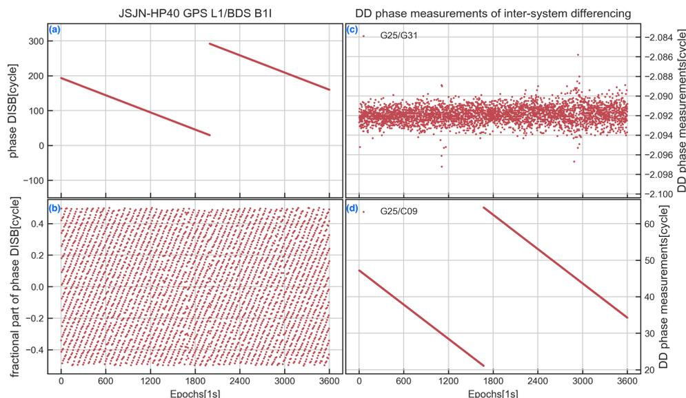
**Figure 9.** Time series of integral part (a) and the fractional part (b) of the phase DISB of GPS L1/BDS-2 B1I, and the DD phase measurements of G25/G31 (c) and G25/C09 (d).
