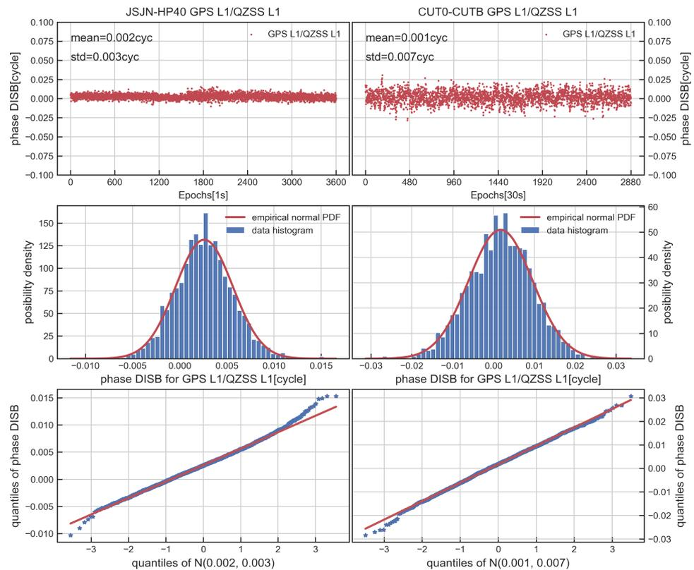
**Figure 7.** Time series, distribution and QQ plot of GPS L1/QZSS L1 phase DISB for JSJN–HP40 (left) and CUT0–CUTB (right).
