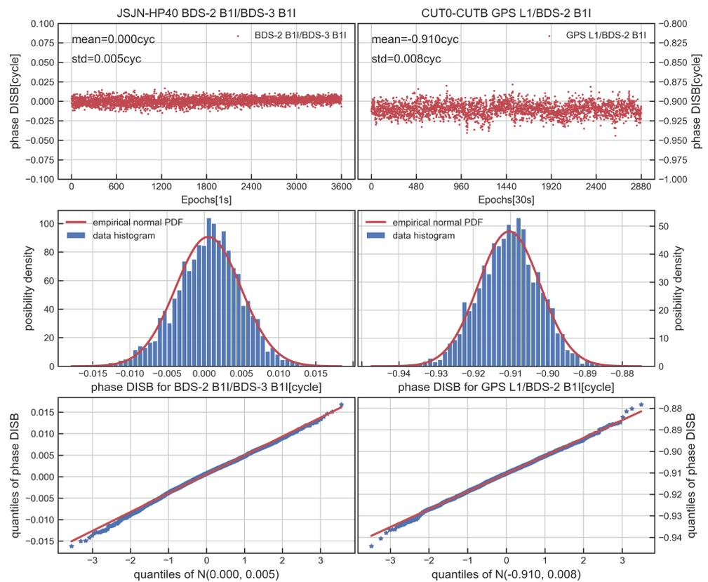
**Figure 8.** Time series, distribution and QQ plot of BDS–2 B1I/BDS–3 B1I phase DISB for JSJN–HP40 (left) and GPS L1/BDS–2 B1I phase DISB for CUT0–CUTB (right).
