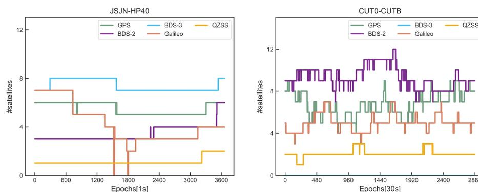
**Figure 2.** Total number of tracked GPS/BDS-2/BDS-3/Galileo/QZSS satellites for the two static baselines datasets.
