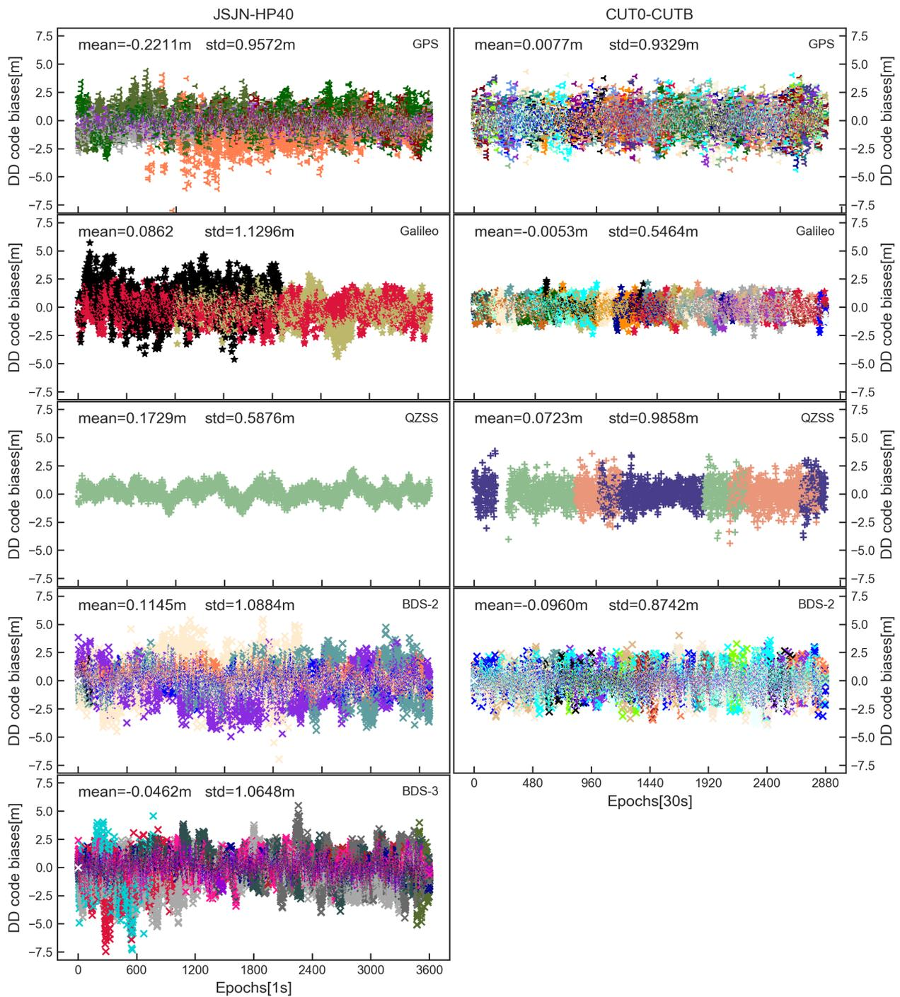
**Figure 4.** The DD receiver channel–dependent code bias (m) of different systems and satellites for JSJN–HP40 and CUT0–CUTB.
