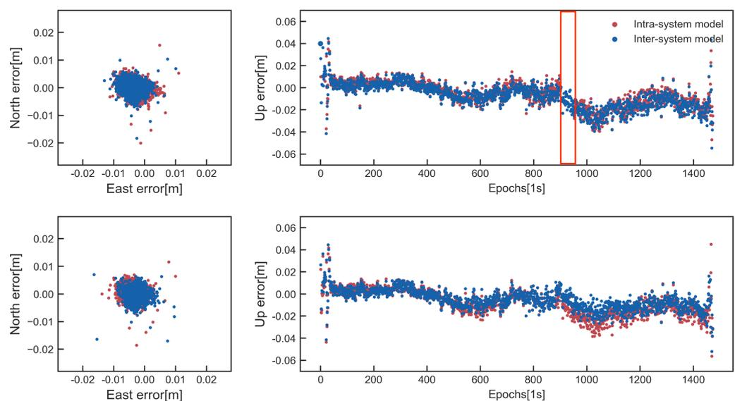
**Figure 12.** Horizontal position scatter and corresponding vertical time series for the intra-system model (red dots) and the inter-system model (blue dots) for the case of GPS + 3 Galileo (top) and GPS + 4 Galileo (bottom).
