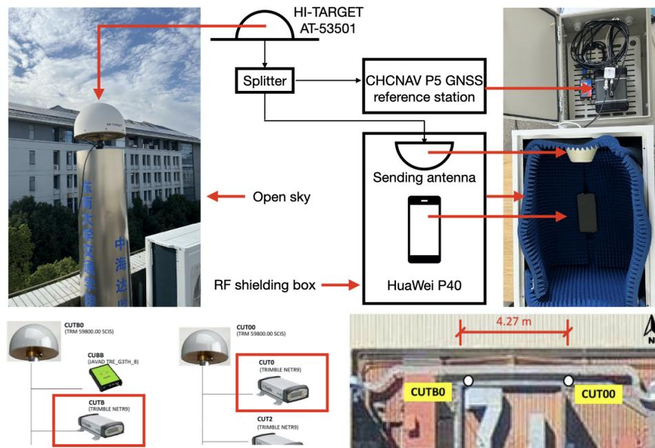
Figure 1. Layout of the smartphone and receiver for two static baselines.
