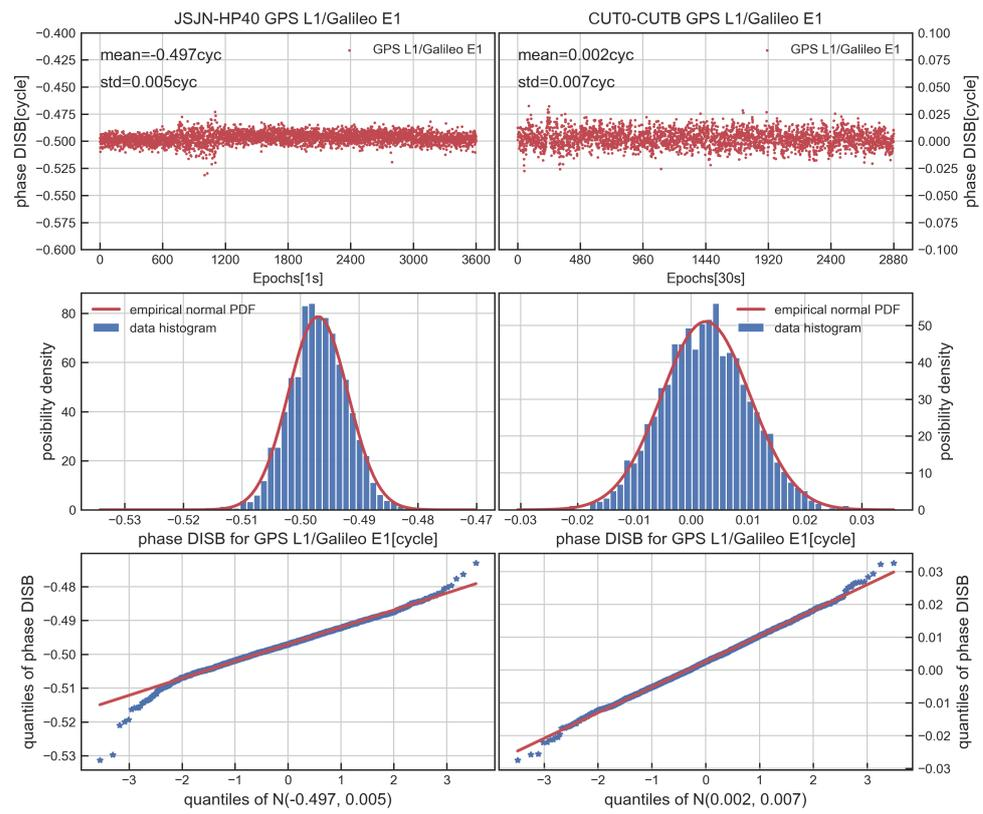
**Figure 6.** Time series, distribution and QQ plot of GPS L1/Galileo E1 phase DISB for JSJN–HP40 (left) and CUT0–CUTB (right).
