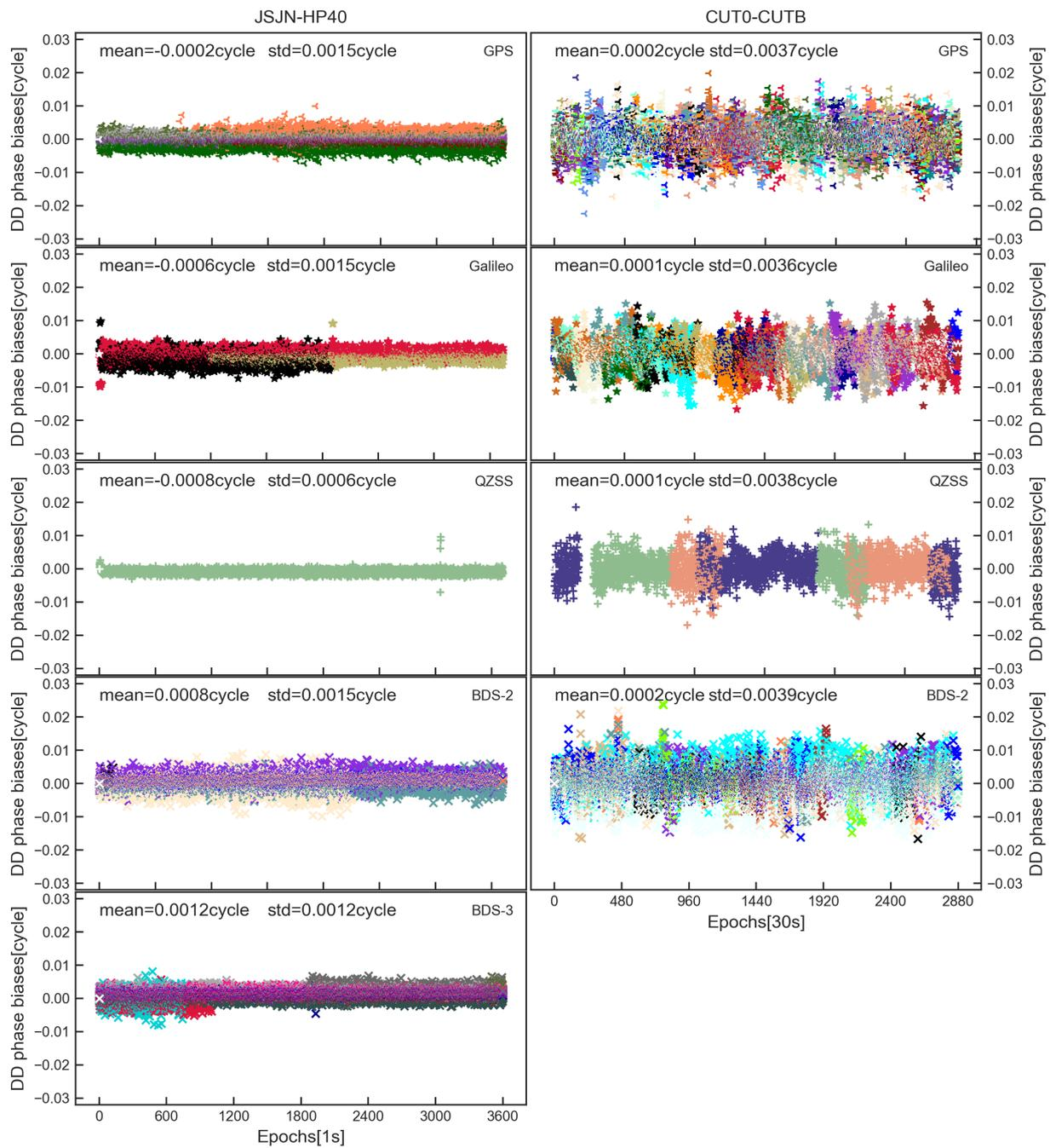
**Figure 3.** The DD receiver channel–dependent phase bias (cycle) of different systems and satellites for JSJN–HP40 and CUT0–CUTB.
