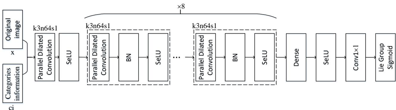
**Figure 4.** Network structure of the discriminator. K, n, and s indicate kernel size, number of feature maps, and stride, respectively.
