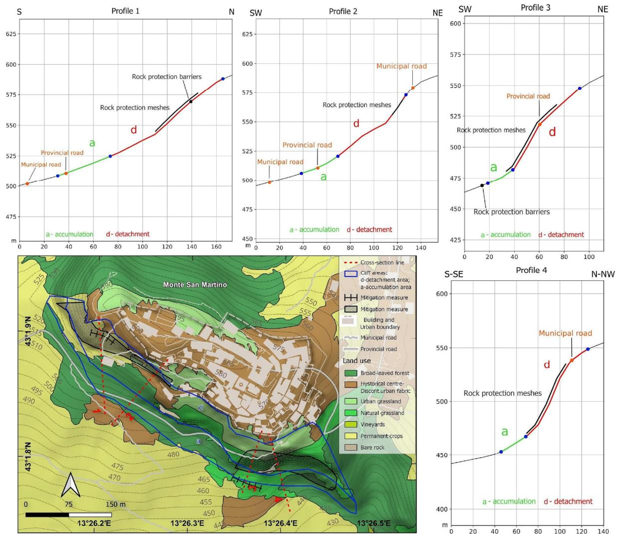
**Figure 12.** Location of the slopes' safety works superimposed on the land use (land use map of the Marche Region at the scale of 1:10,000) in Monte San Martino. The outlines of the four most representative profiles shown in the figure are also traced.
