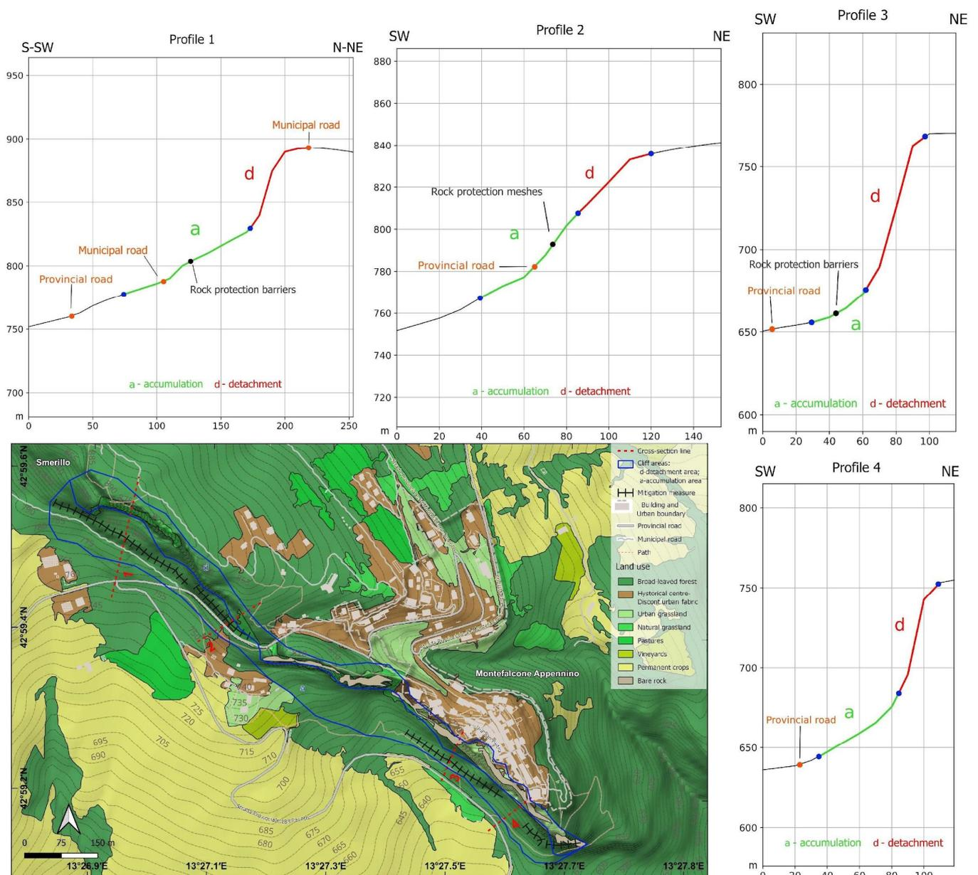
**Figure 11.** Location of the slopes’ safety works superimposed on the land use (land use map of the Marche Region at the scale of 1:10,000) in Montefalcone Appennino. The outlines of the four most representative profiles shown in the figure are also traced.
