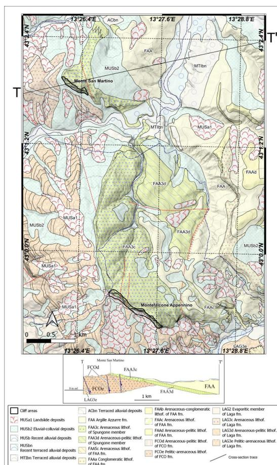
**Figure 2.** Geological map reduced in scale (1:25,000) from the Marche Region’s 1:10,000 scale geological cartography with a cross-section modified from Sheet 314 [16] of the geologic map of Italy, showing the general structural attitude of the Pliocene sedimentary body that forms the studied cliffs.
