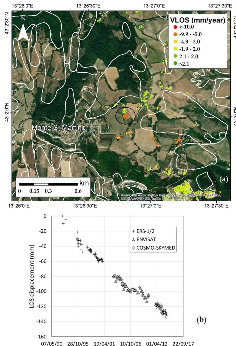
**Figure 14.** VLOS (mm/year) for the period from 2011 to 2014 acquired by the COSMO-SkyMed ascending satellite in the area of Monte San Martino. The white lines represent the landslides mapped via the PAI. (b) LOS displacement time series of the movements detected in proximity to the village. The location of the measuring points is shown as a black circle in (a).
