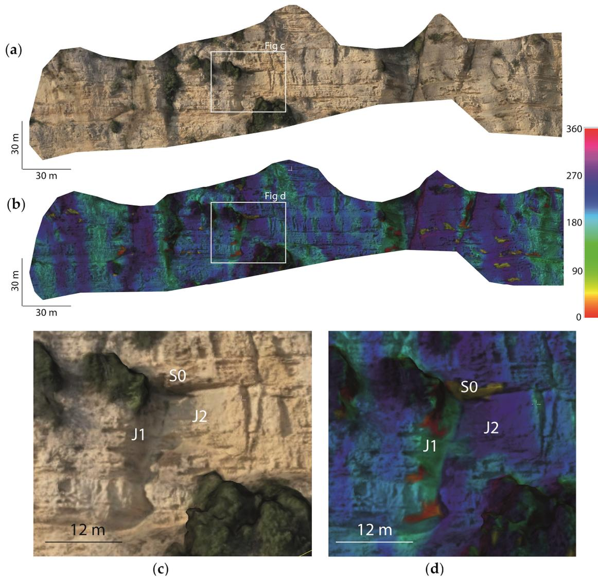
**Figure 13.** (a) 3D model of the cliff in RGB colors. (b) Three-dimensional model of the cliff, with the dip directions of the slope faces (and joints) highlighted. (c) Sector of the slope where the intersection of S0, J1 and J2 brought about the detachment of a large rock block. (d) The same sector as shown in (c) with the dip directions of the slope faces (and joints) highlighted.
