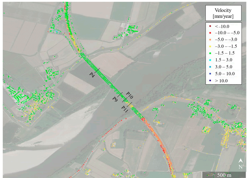
Figure 10. Distribution of the PSs identified in the case-study area illustrated in a colour scale representing their displacement velocity along the satellite LoS.
