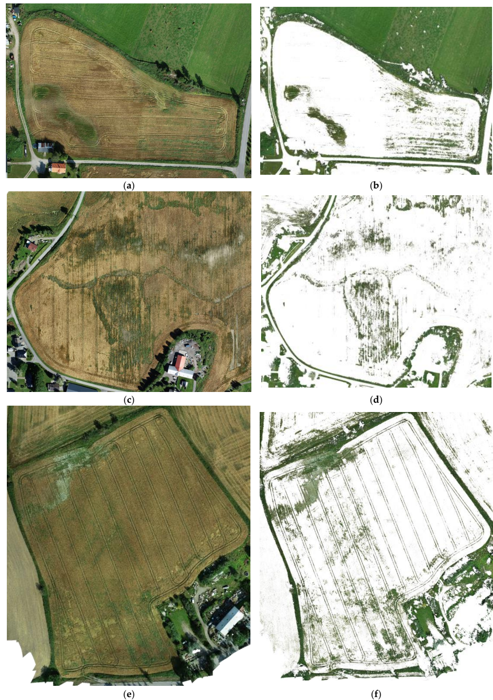
Figure 9. Examples of original UAV image (a,c,e) and predicted output weed map (b,d,f) with the cereal crop masked (white pixels) using the DL model 1DTransformer. Green vegetation outside the cereal fields was also detected as weeds.
