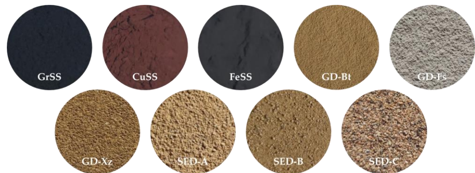
Figure 3. Physical images of aerosol particle samples. GrSS, CuSS, and FeSS, respectively, represent the graphite, copper powder, and iron powder smoke screen samples; GD-Bt, GD-Fs, and GD-Xz, respectively, represent the ground dust samples collected from Baotou City, Fangshan District, and Xuzhou City, with soil types of loam, silt, and silt loam; SED-A, SED-B, and SED-C, respectively, represent the soil explosion dust samples collected from explosives blasted in silt, silt loam, and sandy loam.
