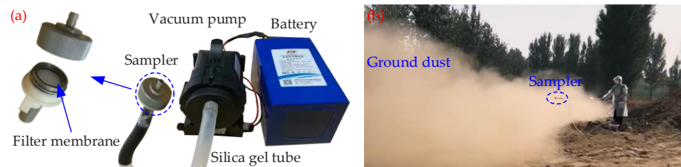
Figure 1. Ground dust sampling: (a) physical diagram of ground dust sampling device; (b) real scene of ground dust sampling.
