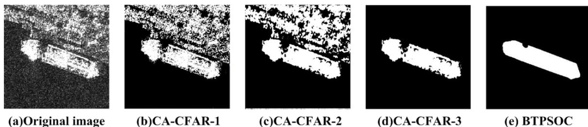
**Figure 16.** Experiment result comparison of the CA-CFAR and BTPSOC algorithms.
