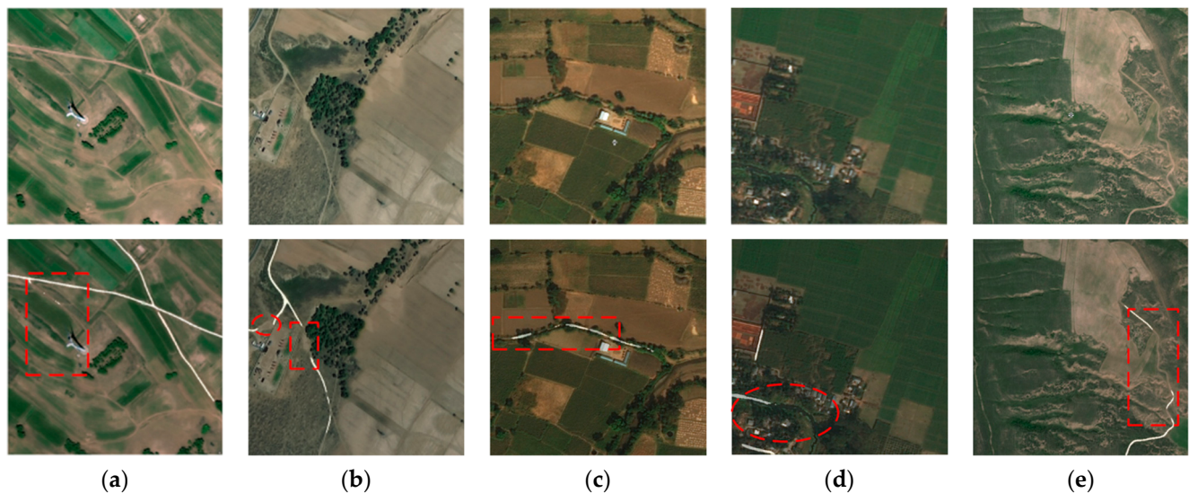
Figure 1. Characteristics of sandy roads and challenges in extraction. These images illustrate the difficulties in the extraction process and the characteristics of sandy roads. The first row comprises representative original images from the sandy road dataset, and the second row consists of the resultant images obtained from the extraction of the U-Net network model. The areas outlined in red represent road segments that have not been correctly extracted, due to the following reasons: (a) Roads are confused with bare soil boundaries. (b) Roads have poor continuity and blurred sections in between. (c) Roads are obscured by trees. (d) Streams are incorrectly extracted as roads. (e) Roads contain distinctive banding features.
